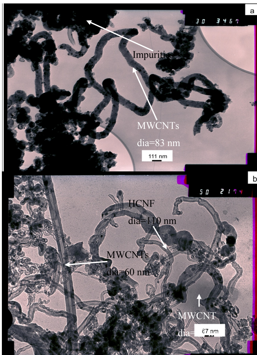
Figure 4.16: Electron micrographs obtained at 20 minutes, 850 °C temperature, 594 ml/min C 2 H 2 flowrate and 2 g catalyst. (a) consists of MWCNTs while (b) consists of MWCNTs and HCNFs.
