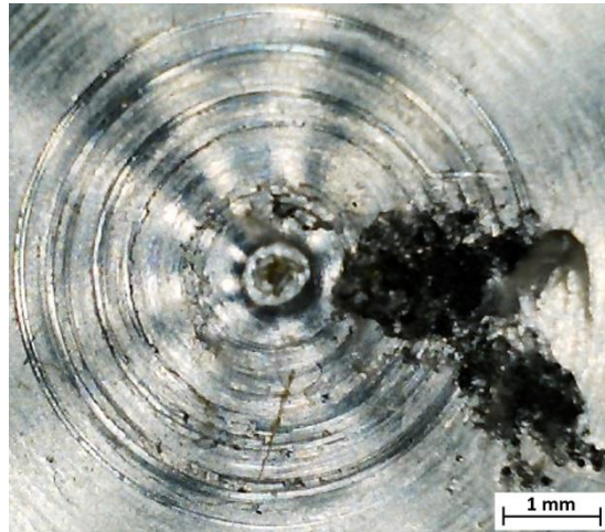
Fig. 4.52: Striations made by DB4.
