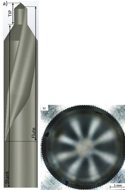
Fig. 3.7: a) CAD model of drill bit and b) diagram indicating a perfect circle fitted to a hole drilled by the purchased drill bit.
