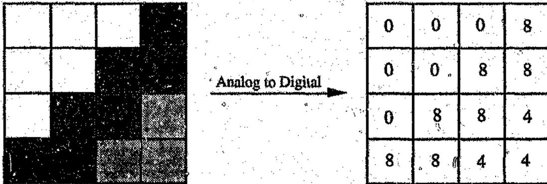
Figure 2 - Digital representation of an analog image
