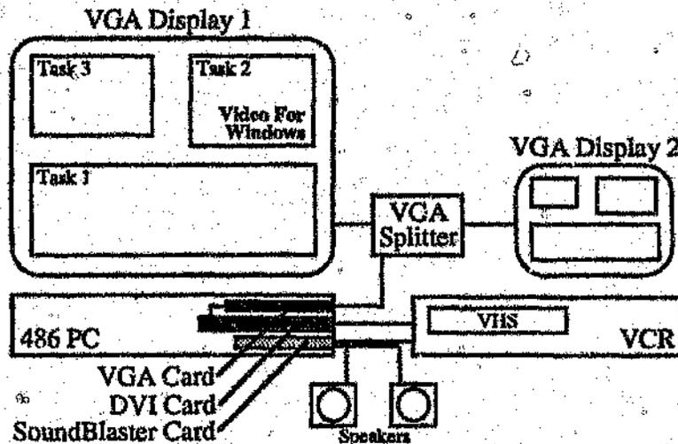
Figure 4 - The components of the experiment
