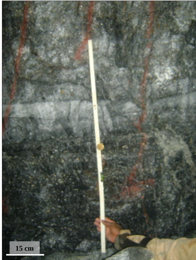
Figure 3.11: The Vaal Reef A Facies at the 500 geozone at Moab Khotsong Mine. The A Facies is over 1.2 m in thickness showing internal quartzite within the reef.
