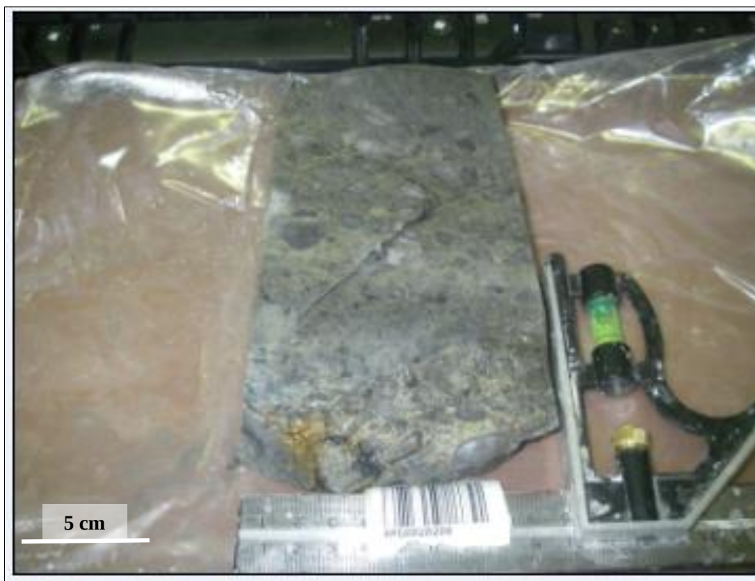
Figure 4.2: Hand specimens from the Vaal Reef C Facies at Kopanang Mine collected from the 440 geozone with high pyrite content with sub-round quartz pebbles.
