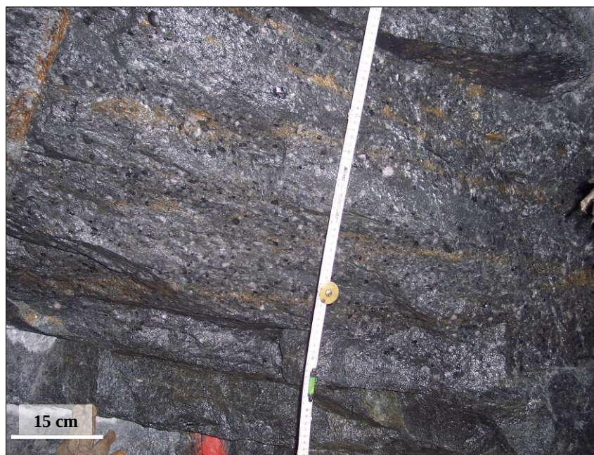
Figure 3.12: The Vaal Reef A Facies in the 370 geozone at Moab Khotsong Mine showing the Almond Reef; the reef overlies the Mizpah quartzite.
