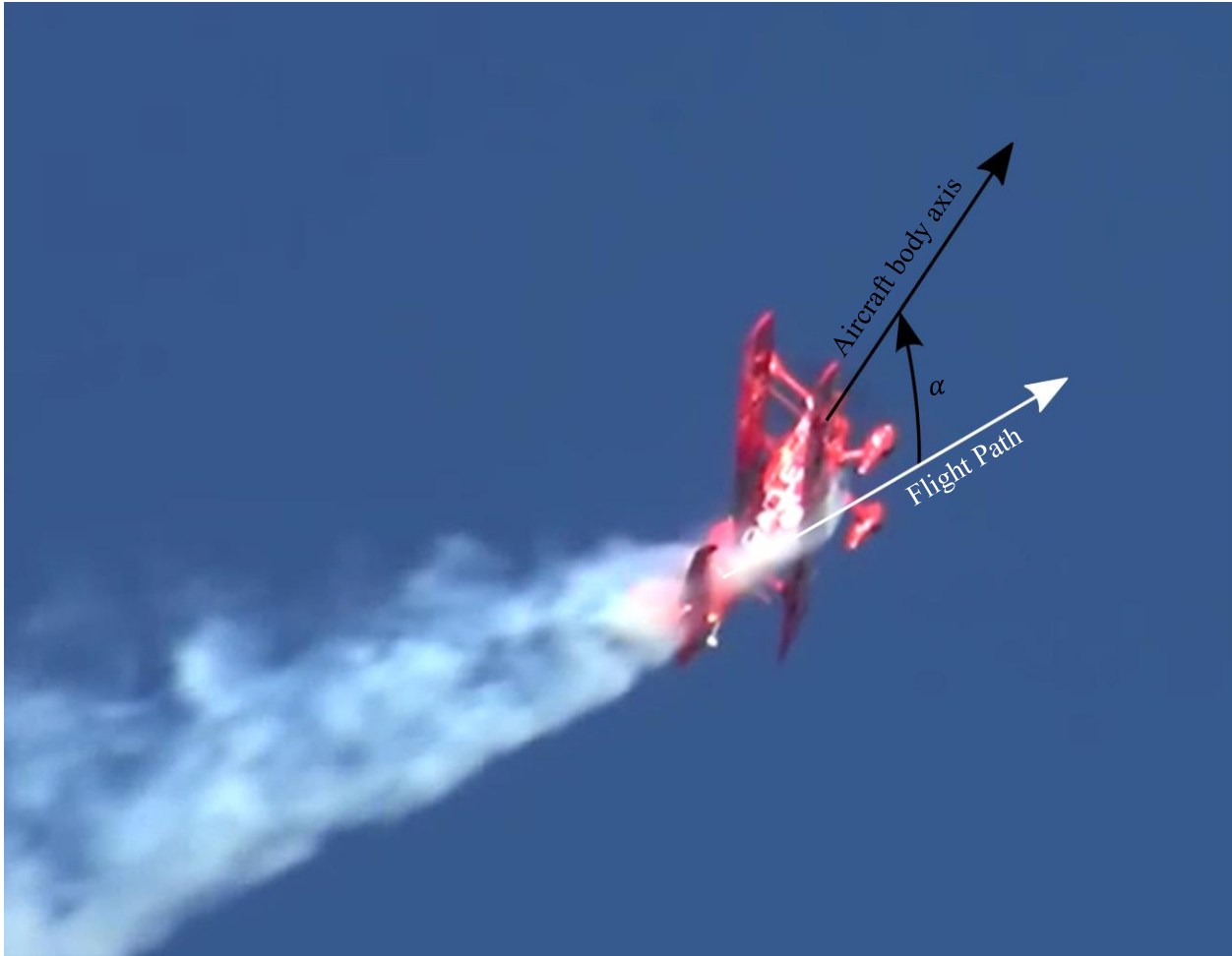
Figure 104: Illustration of high alpha flight during a tumble manoeuvre
