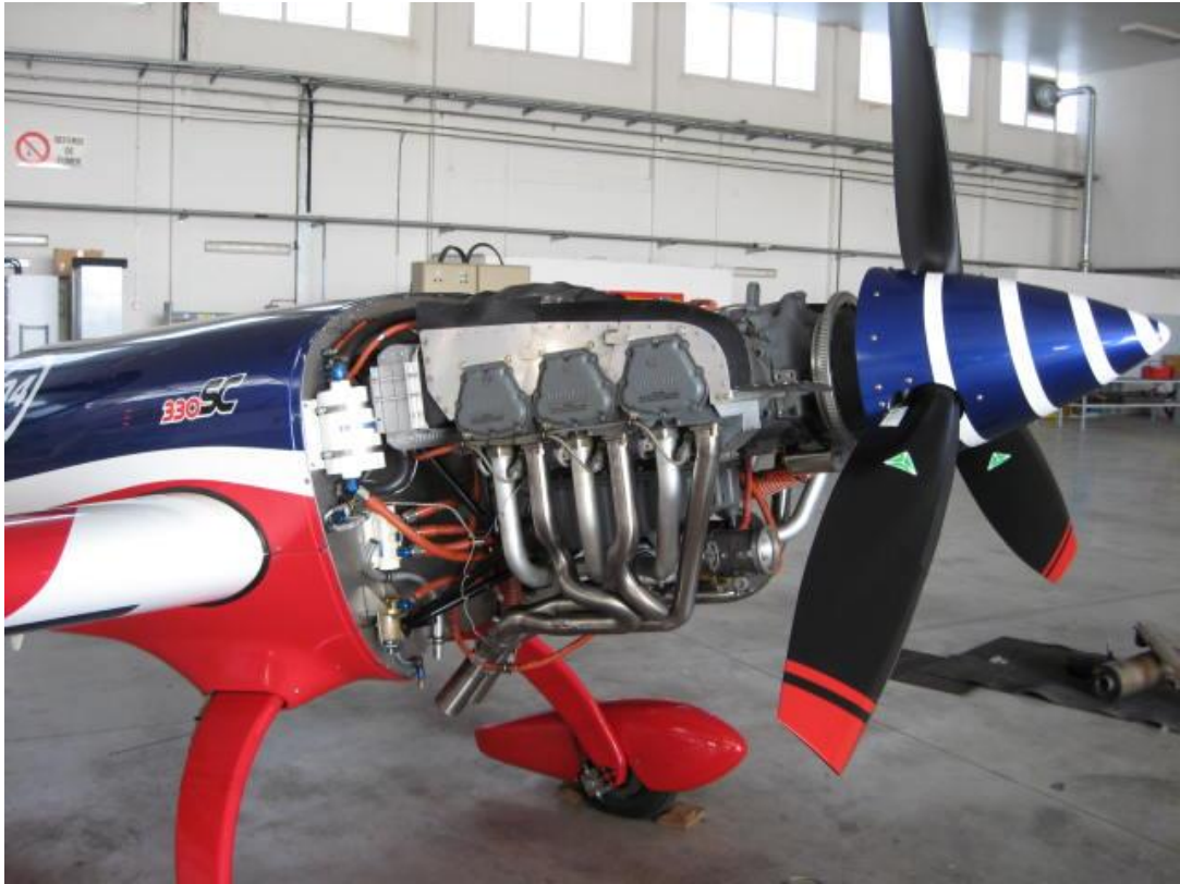
Figure 59: Extra 330SC exposed engine (installed on airframe) [72]
