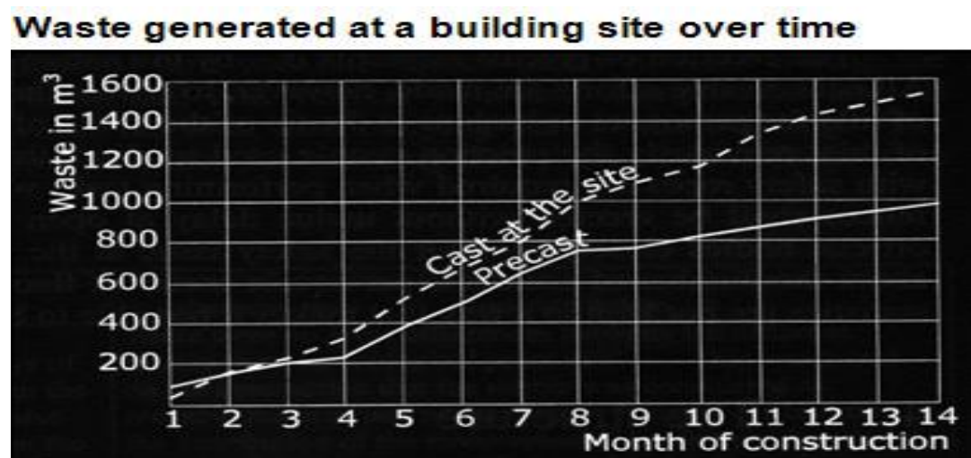
Figure 2.8. Waste generated at a construction site (CPCI, 2012)
