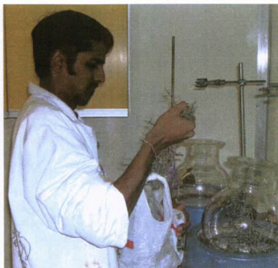
Figure 2.1. Freshly collected plant material was cut up and the essential oil was collected by steam distillation using a Clevenger apparatus.
