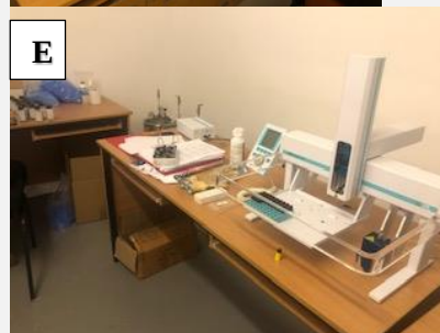
Figure 4-1: A-B Preparation of sampling equipment (Hach HQ40D Multi Meter Kit). Boreholes are installed with a solar-powered pump. The valve at the top of the borehole was opened with a wrench. An electrical contact gauge was used to measure the water level C. Sampling from a well with a bucket pulley. D-E. LGR Isotope Analyzer at the UNAM Laboratory in Windhoek F. Stable isotope samples being injected into the tray for analyses.
