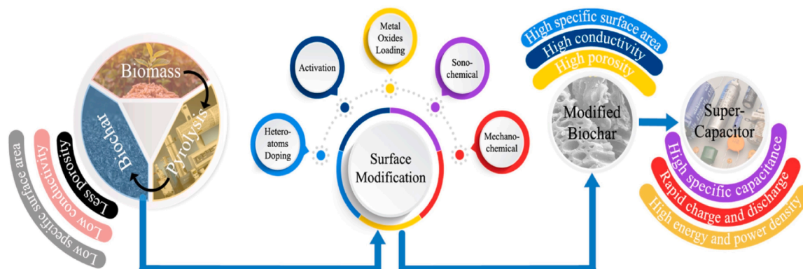
Fig. 5. Schematic illustration of modifying biochar for supercapacitor applications. Reproduced with permission from ref (mehdi et al., 2022). Copyright 2022 MDPI.
