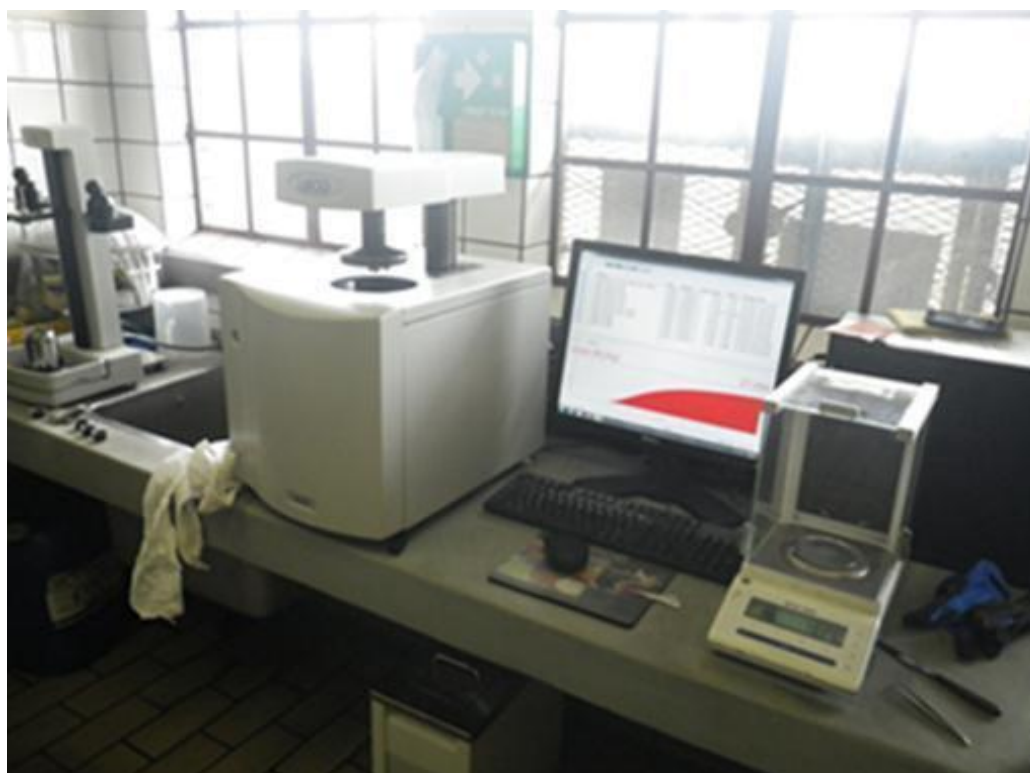
Figure 3.10: CV Calorimeter for determination of heat value (MJ/kg)
