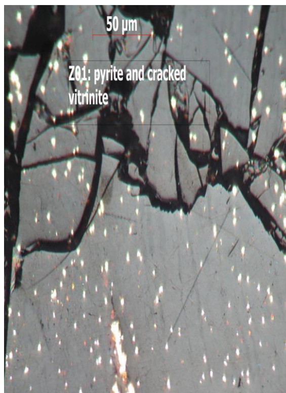
Figure 4.42: Sample Z01 showing pyrite and cracked vitrinite
