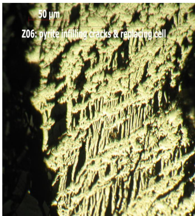
Figure 4.43: Sample Z06 showing pyrite infilling cracks
