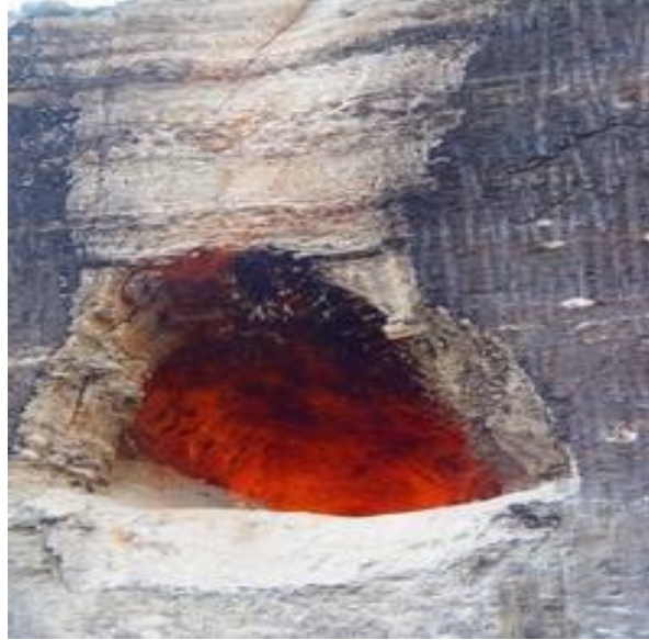
Figure 1.19: Burn zone around a mine addit due to sponcom
