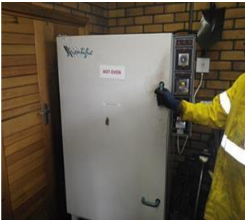
Figure 3.9: Drying oven for sample preparation at 105 °C
