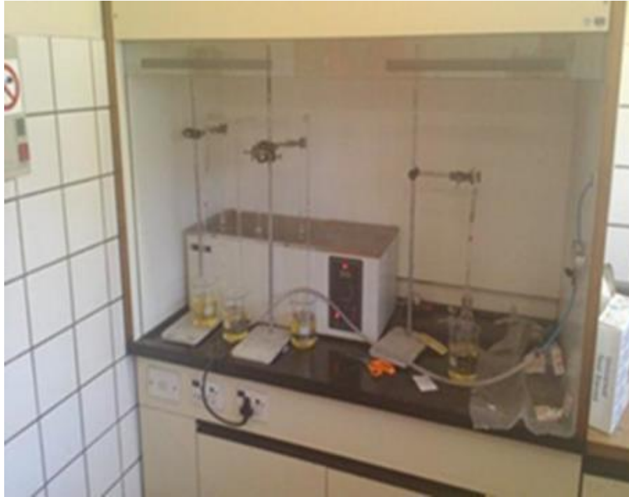
Figure 3.7: Oxygen adsorption test apparatus at mine laboratory
