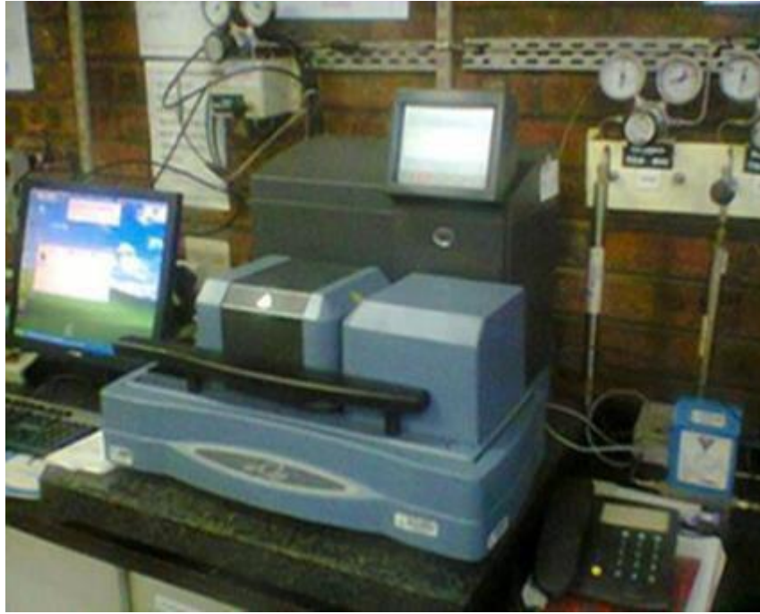
Figure 3.6: TGA analyser used at Wits University
