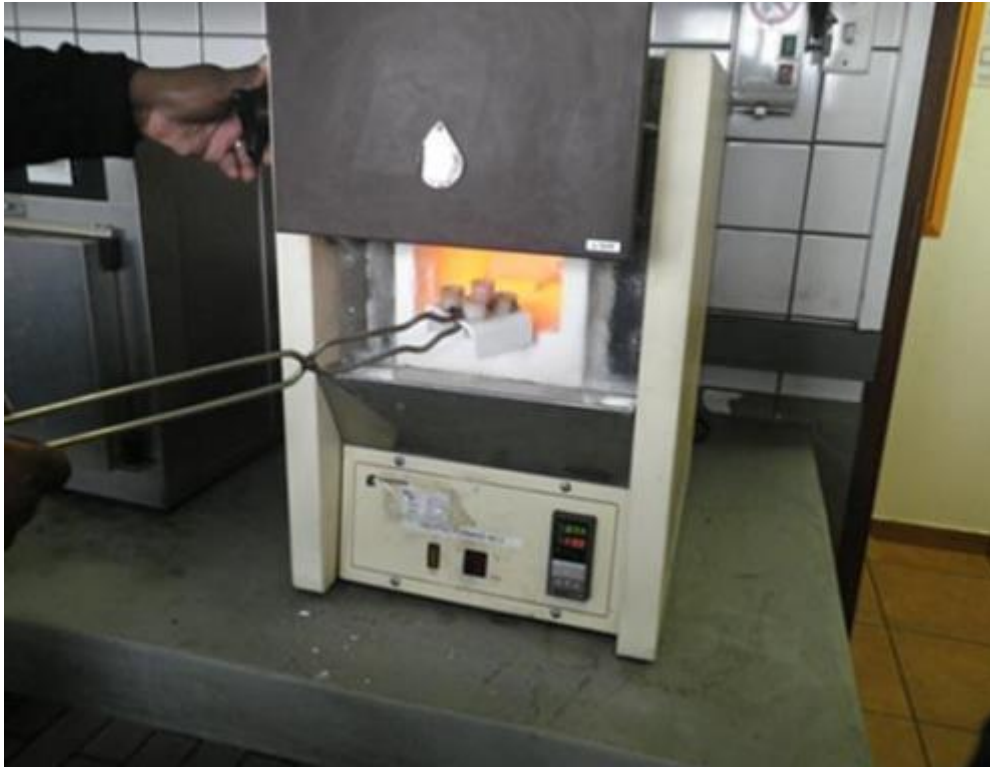
Figure 3.11: Volatile furnace (950 °C)
