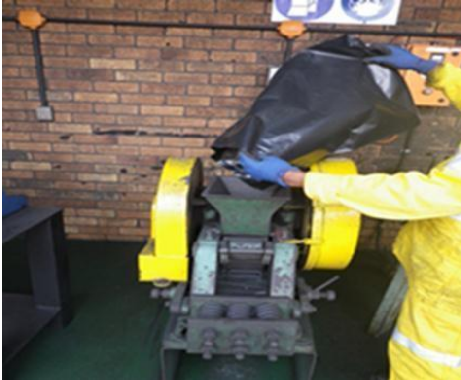
Figure 3.3: Crushing of drill-cores to 20mm top size
