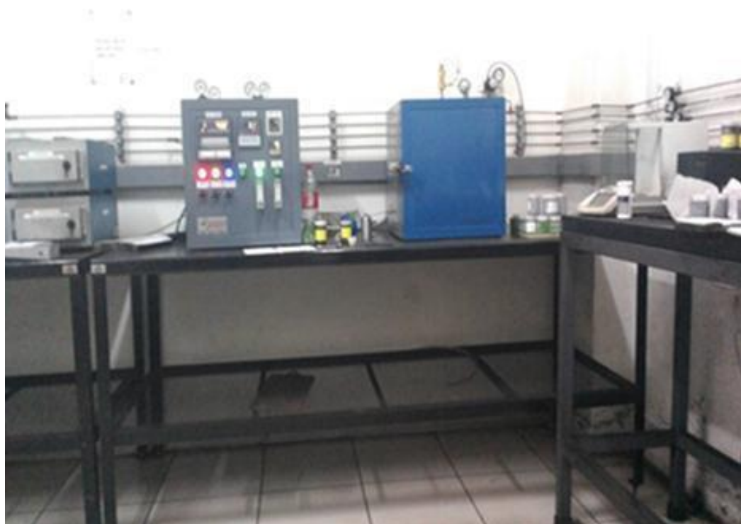
Figure 3.4: Crossing point temperature instrument with control unit and furnace
