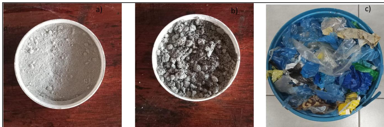
Figure 4.2: As received a) coal fly ash, b) coal bottom ash, and c) low density polyethylene.
