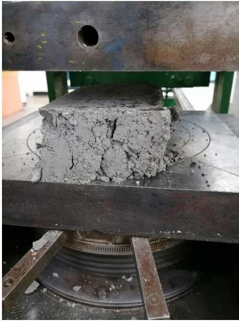
Figure 5.7: Stress beyond load of failure applied on the 0.05 wt.% CNT brick
