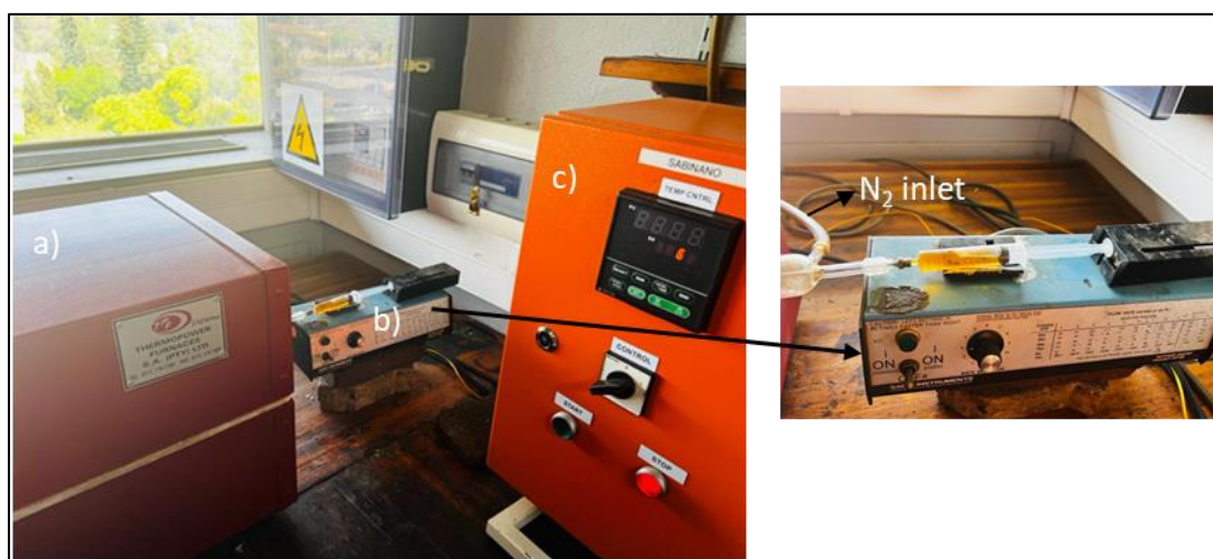
Figure 3.1: FCCVD reaction setup a) horizontal furnace, b) syringe pump, and c) temperature control system
