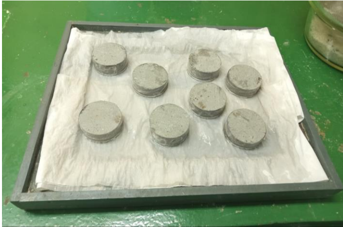
Figure 6.4: Sorptivity tray with specimens and Ca(OH) 2 solution
