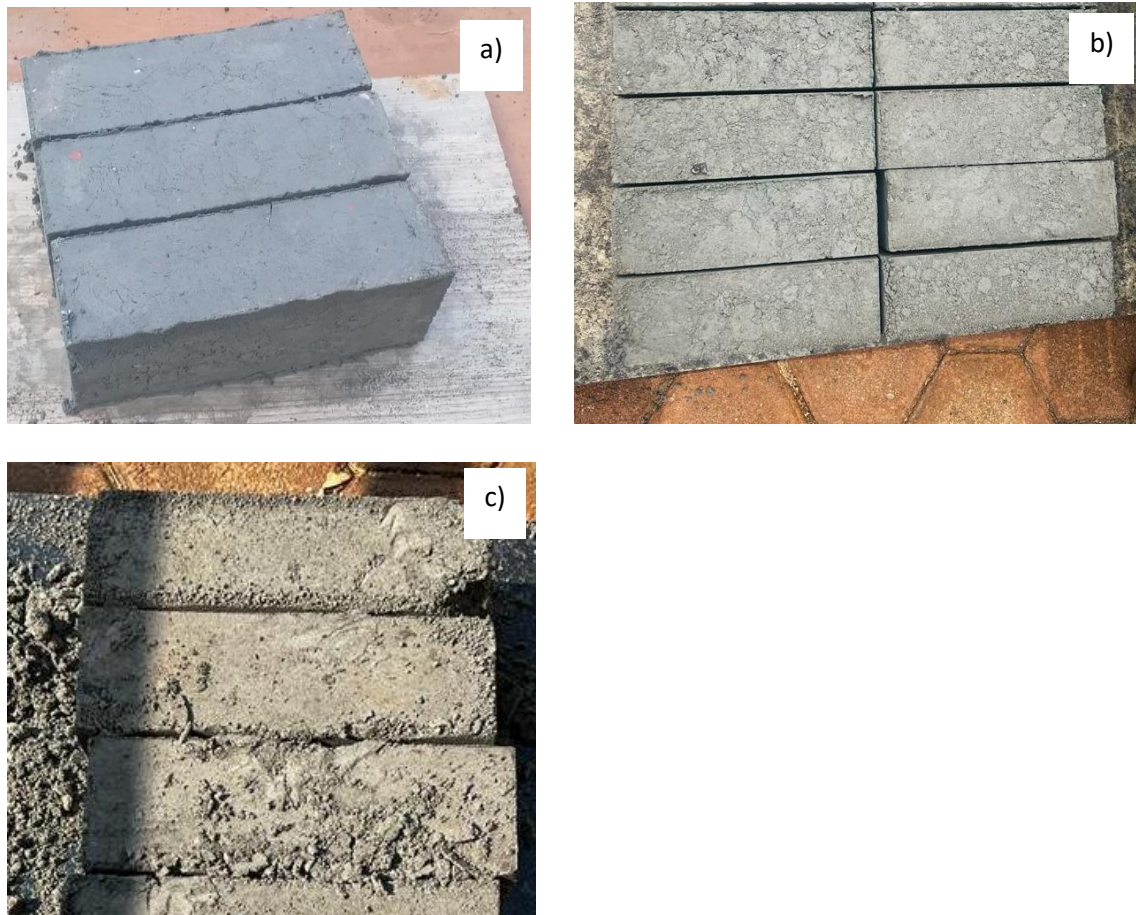
Figure 5.3: Brick samples using different coal fly ash : LPDE ratios. a) 80:20, b) 85:15 and c) 90:10.
