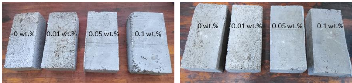
Figure 6.13: Control, 0.01, 0.05 and 0.1 wt.% CNT bricks before and after efflorescence tests
