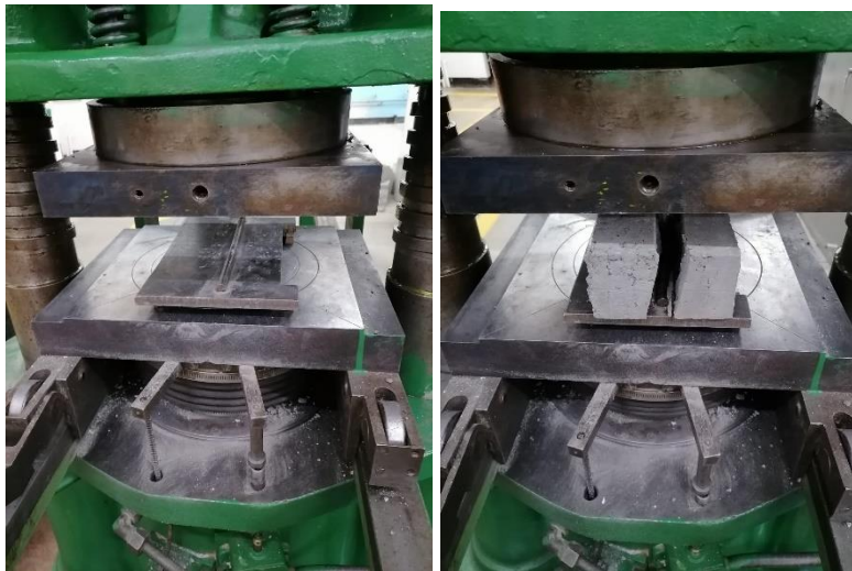
Figure 5.2: Split tensile strength testing setup
