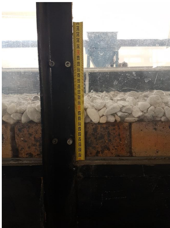
Figure 3-3: Section of Flume C with clear Perspex and measuring tape for measuring flow depths.
