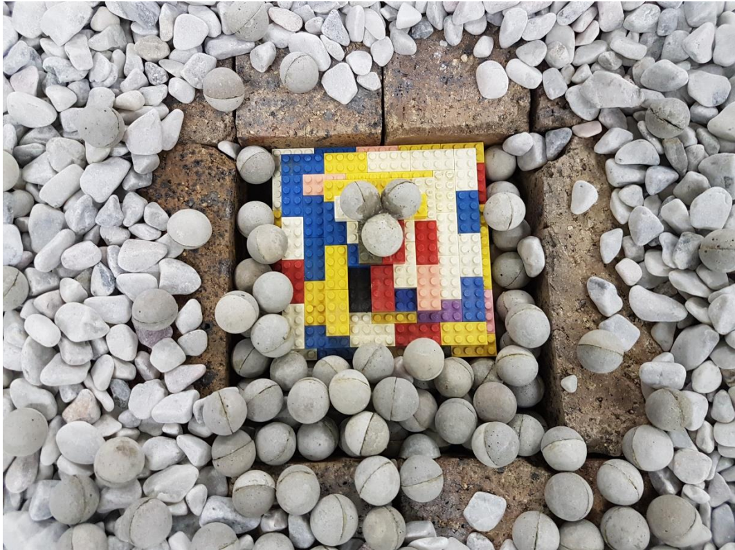
Figure 3-5: Lego brick used to alter the depth of the boulder; Triangular base of 3 spheres for boulders to rest on.
