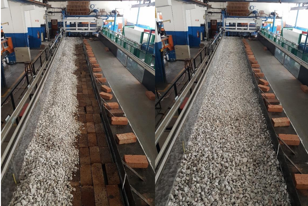
Figure 3-4: Flume C lined with bricks and pebbles to create artificially raised bed.
