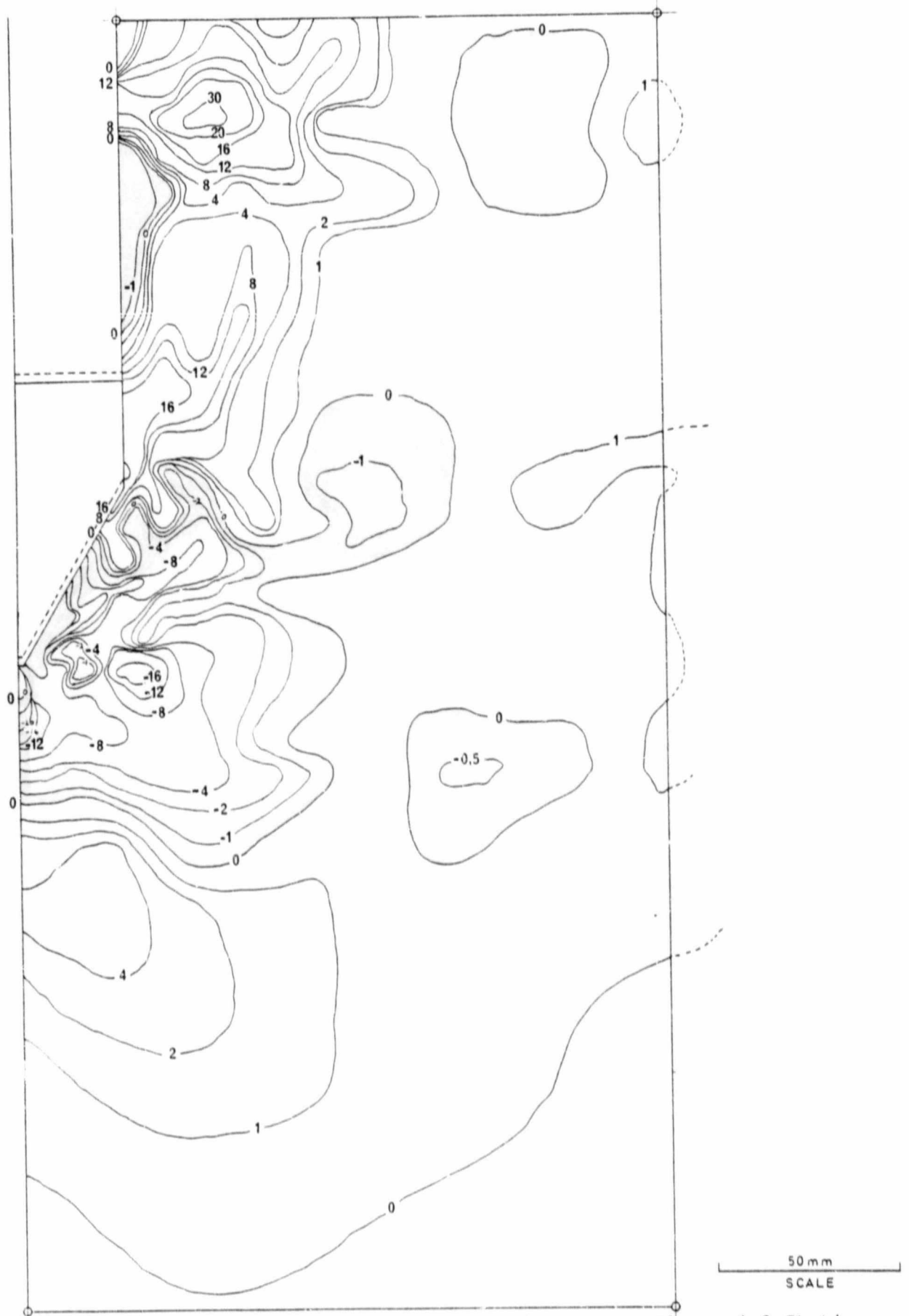
FIGURE 6.32 Volumetric strain contours at 10^3 \mu -strain. Plates 1-3 Static.
