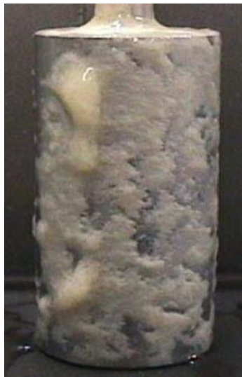
Figure 3.7: Stainless steel cylinder covered with biofilm after 7 days of growth (Simões, 2005 page 167)
