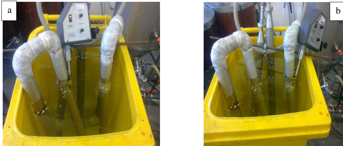
Figure 3.11: Arrangement during use of ultrasound waves for run 1 on (a) pipe C and (b) pipe D before swabbing. NB: sonication device as fastened to pipes using jubilee clamps
