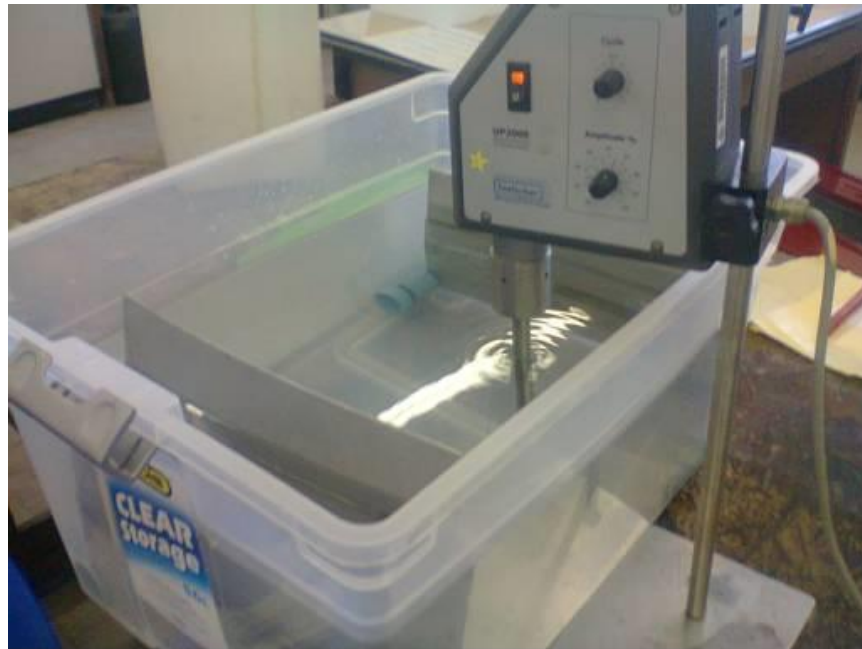
Figure 3.2: Experimental setup and procedure using ultrasound waves to control biofilms from SS coupons
