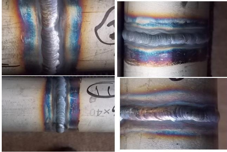
Figure 4.27: Photographs of weld caps of 50 mm ID, 3.91 mm wall thickness, 316L pipe apparatus conducted at SAIW using TIG welding and using 316L and 904L filler rods
