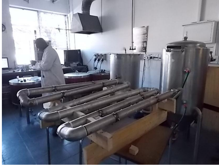
Figure 3.5: Test rig to investigate the effect of biofilm formation after CIP on brewing process systems
