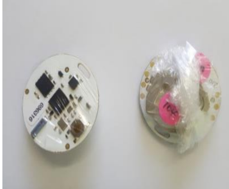
Figure B.1: Proximity tags covered in plastic for protection
