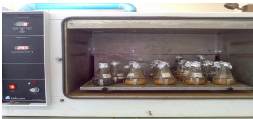
Figure 3.2. Agitation leaching test equipment (Labcon shaking incubator)
