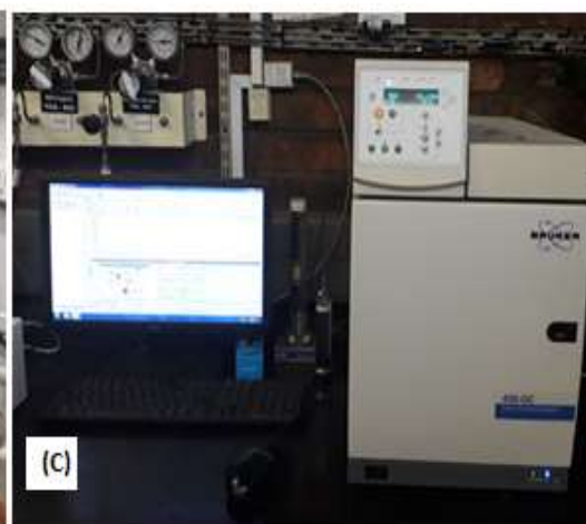
Figure 3.4: Pictures of the mixed gas permeation apparatus at WITs [A – Full view of the equipment. B – Oven that housed the membrane module. C – Gas chromatography]
