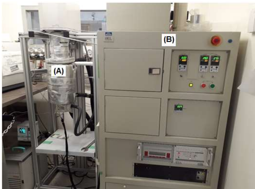
Figure 3.5: Picture of the gravimetric sorption analyzer at UoM [A- sample chamber, B- control panel]
