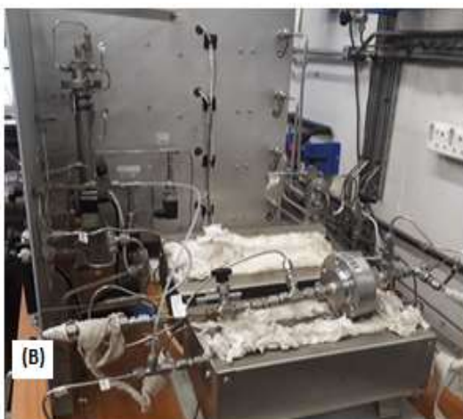
Figure 3.4: Pictures of the mixed gas permeation apparatus at WITs [A – Full view of the equipment. B – Oven that housed the membrane module. C – Gas chromatography]
