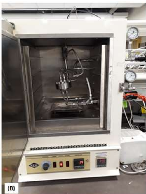
Figure 3.3: Pictures of the mixed gas permeation apparatus at UoM [A – Full view of the equipment. B – Oven that housed the membrane module. C – Gas chromatography]
