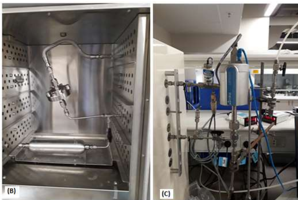
Figure 3.2: Pictures of the pure gas permeation apparatus at UoM [A – Full view of the equipment. B – Oven that housed the membrane module and permeate sample cylinder. C – Close view of e-Baratron digital manometer]
