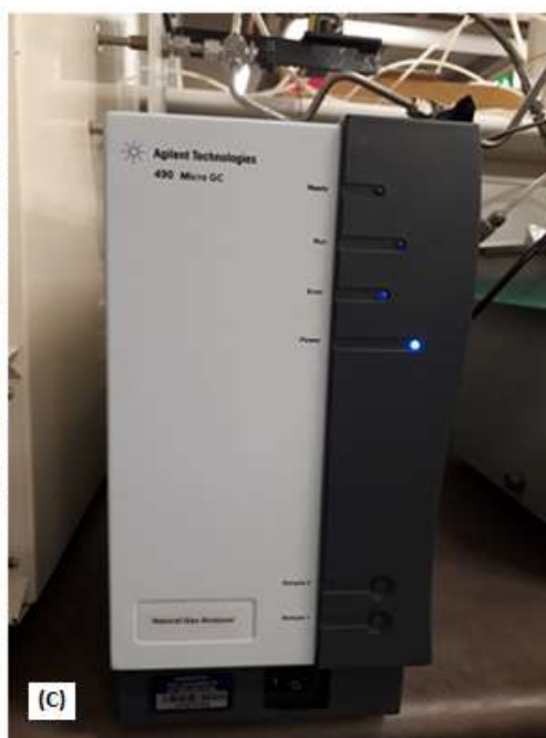
Figure 3.3: Pictures of the mixed gas permeation apparatus at UoM [A – Full view of the equipment. B – Oven that housed the membrane module. C – Gas chromatography]
