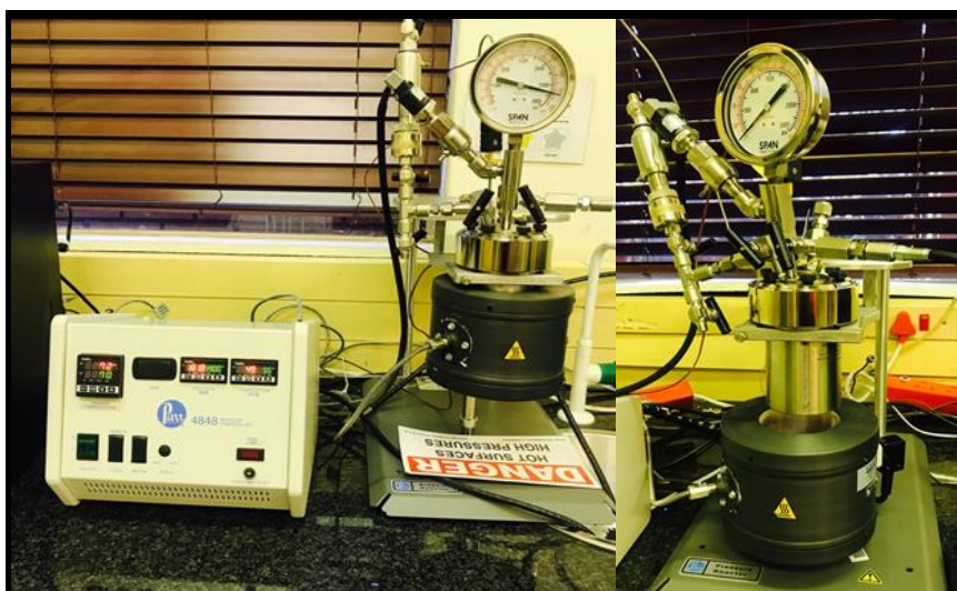
Figure 3.3: N4766 Parr Reactors with controller and heater
