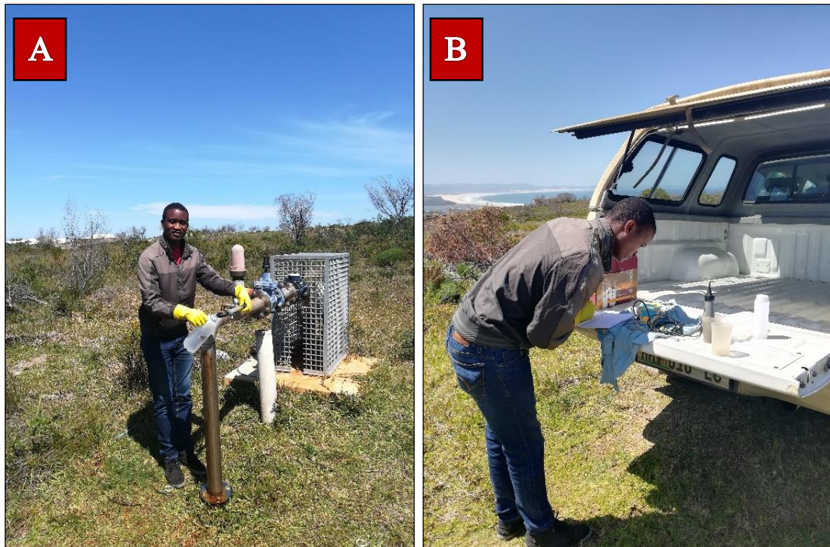
Figure 15: (a, b): Borehole sampling and Field measurements (Eutech Cyberscan PC 10 meter)
