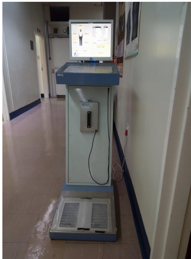
Figure 3.1: Picture showing the CMS60D×D hand-foot-clothes contamination monitor available in the NMD of the CMJAH. This monitor was manufactured by TEMA Sinergie.
