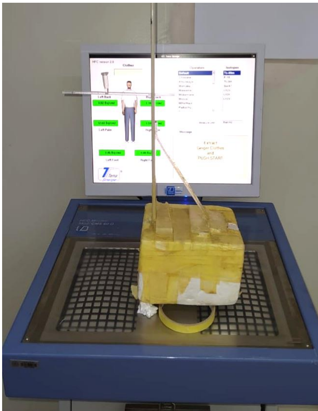
Figure 3.4: Locally made stand ruler source holder placed on top of the contamination monitor.
