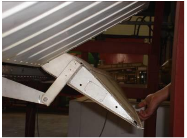
Figure 2. Commonly used external pivot mechanism for single slotted flap systems.
