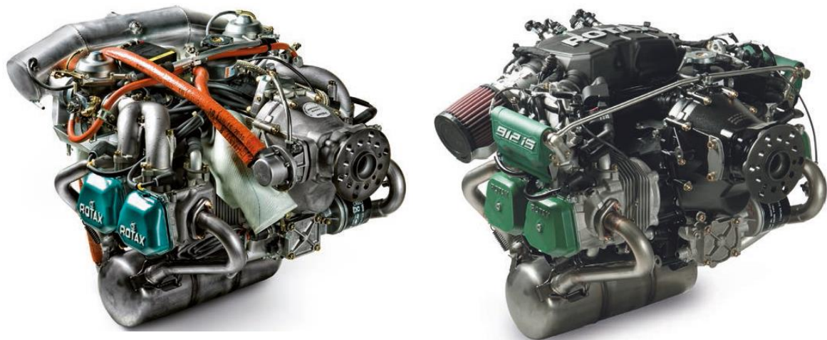
Figure 13. Rotax 912 ULS (left) and 912 iS (right) [25].
