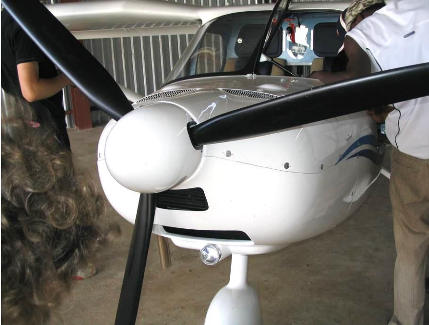
Figure 1: A conventional spinner installed on an aircraft engine.
