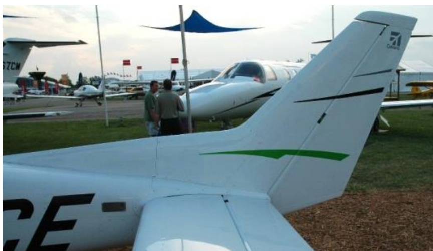
Figure 17. Cessna 162 with increased vertical stabiliser area [author].
