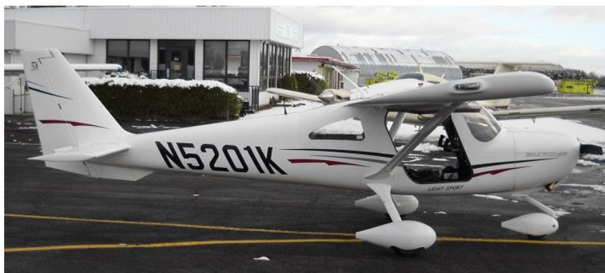
Figure 33. Cessna C-162 indicating strut position and strut sweep [55].
