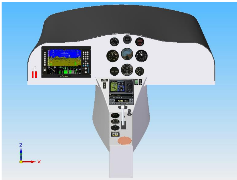
Figure 47. Final instrument panel and console design.
