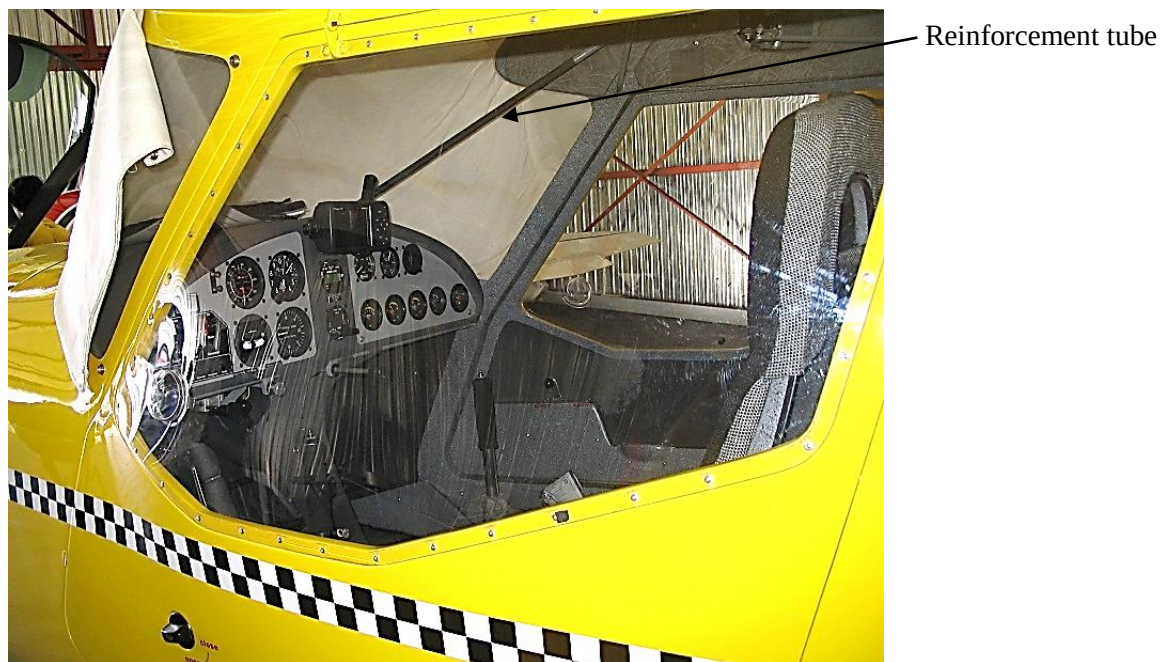
Figure 50. FK-9 cabin with visible reinforcement strut [author].
