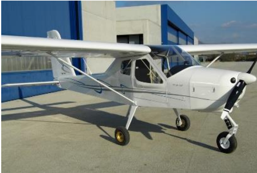
P92 Echo light (500kg) ultralight with simple cowling, straight-leg landing gear and trapezoidal rear window.
