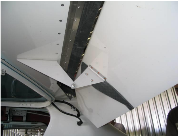
Figure 2. Commonly used external pivot mechanism for single slotted flap systems.
