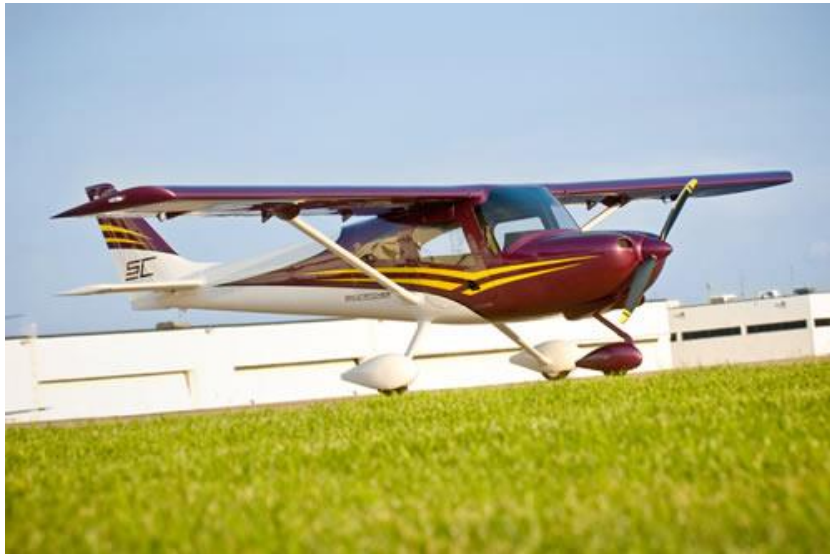
Figure 16. Original Cessna 162 with Rotax 912 engine [36]
