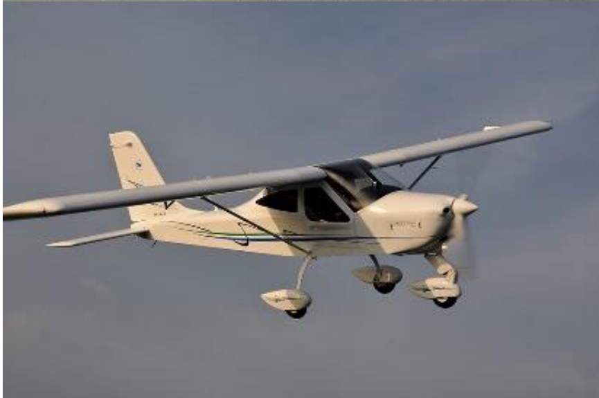
P92 Echo classic (600kg) LSA with a more aesthetic cowling, shrouded nose gear, curved main landing gear leg, vertical tail fillet and triangular rear window.
