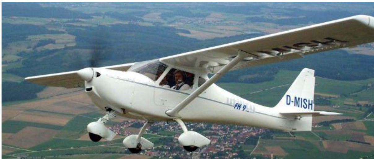
Figure 32. Fk-9 indicating strut position [54].
