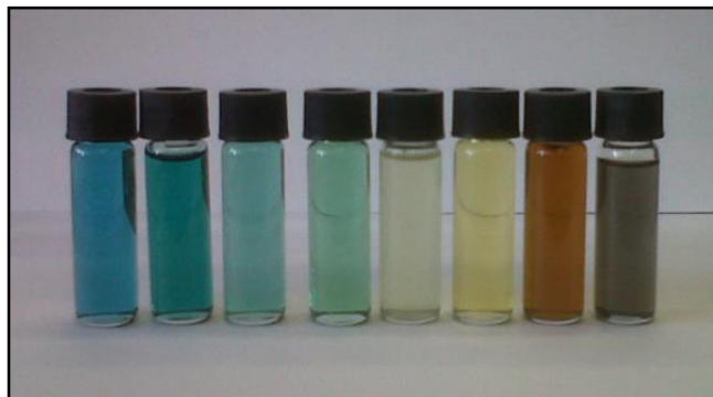
Fig. 3.3.: Size quantization effect in \text{Cu}_2\text{Se} nanocrystals depicted by the change in colour with an increase in time, A being an aliquot at 2 min through to H and aliquot at 60 min.
