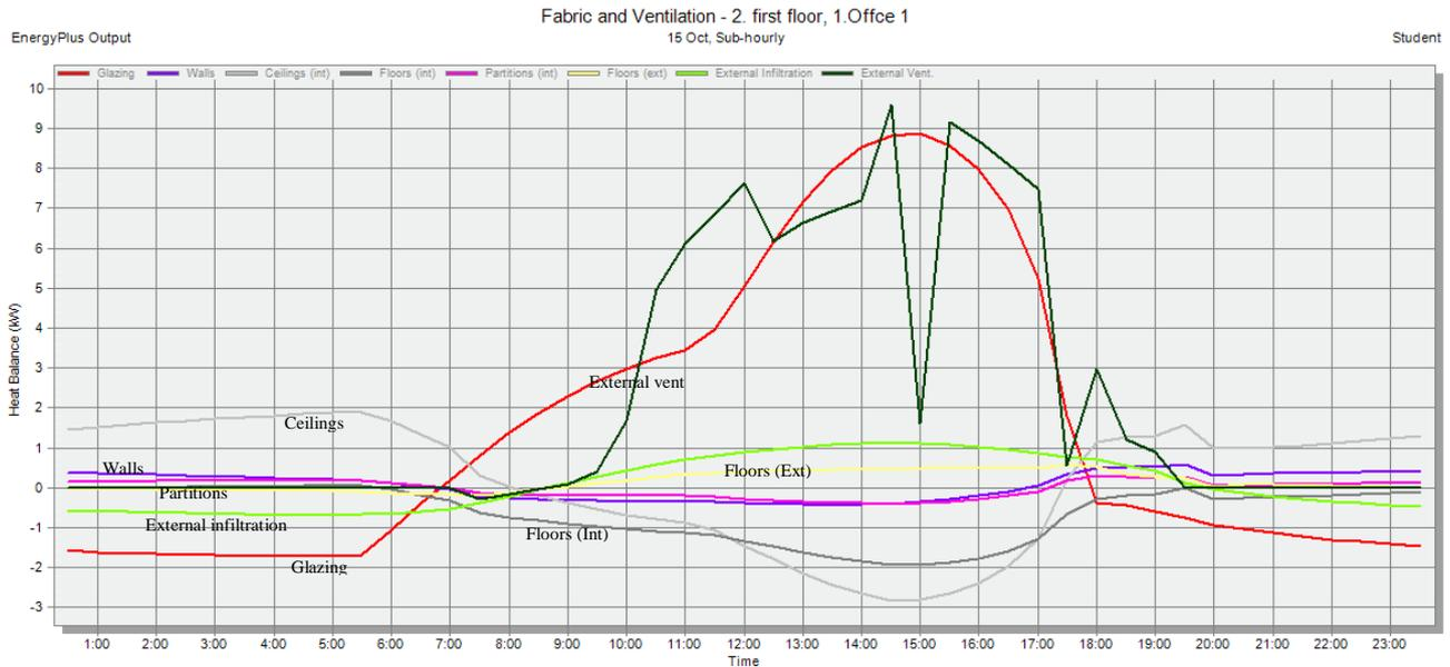
Figure 36: Example of north-eastern facing zone- Office 5 (red line shows glazing -peak 7.15kW & 6.52kWh). Office 8 follows similar profile
