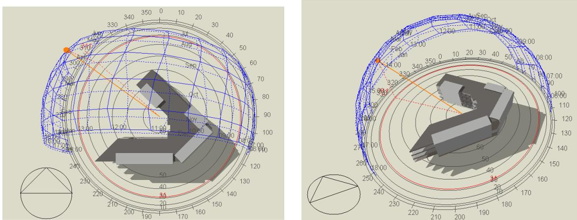
Figure 21: Sun and shadow position at 16th October-plan and axonometric 15pm (summer design day)
