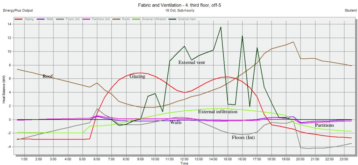
Figure 42: Optimised gains through the roof by insulation (in brown). Office zone 8
