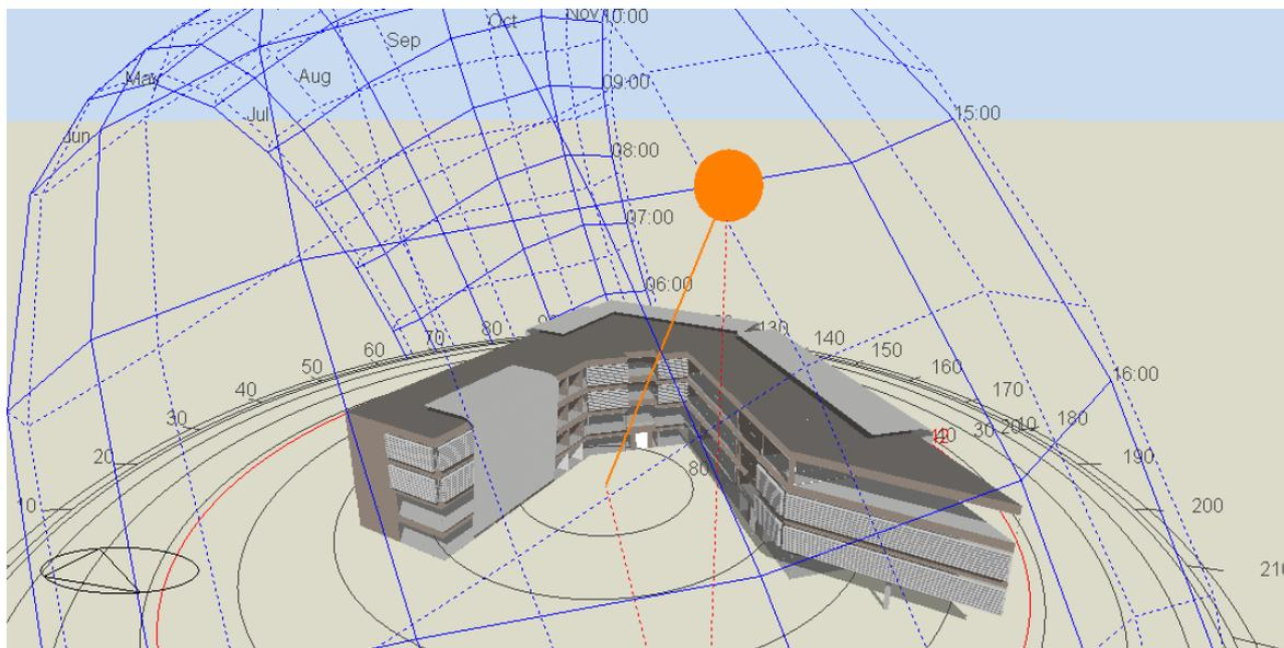
Local shading was selected from DesignBuilder templates for simplicity, permanence and for the fact that it could perform as an aesthetics feature. By modifying the existing template with bespoke model data and trying different options, the following details of the shading were specified in the model for best result over a total window area of 345m<sup>2</sup>.
