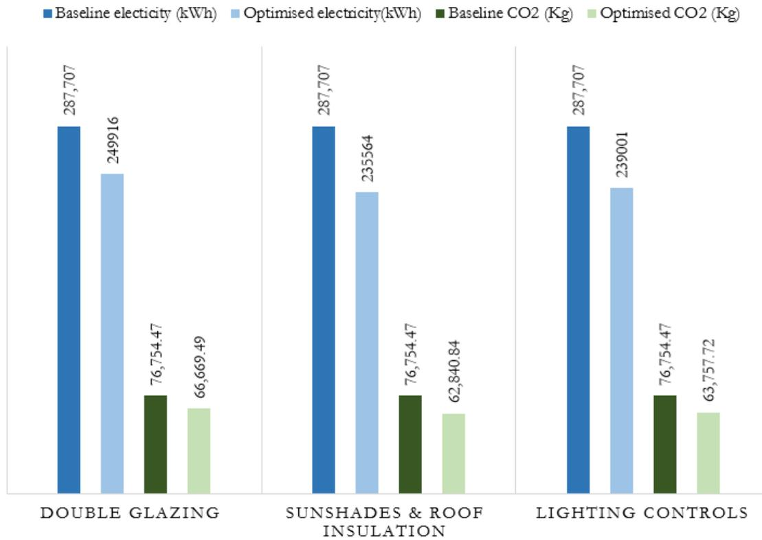
Figure 48: Comparison of savings from the three energy efficiency interventions
