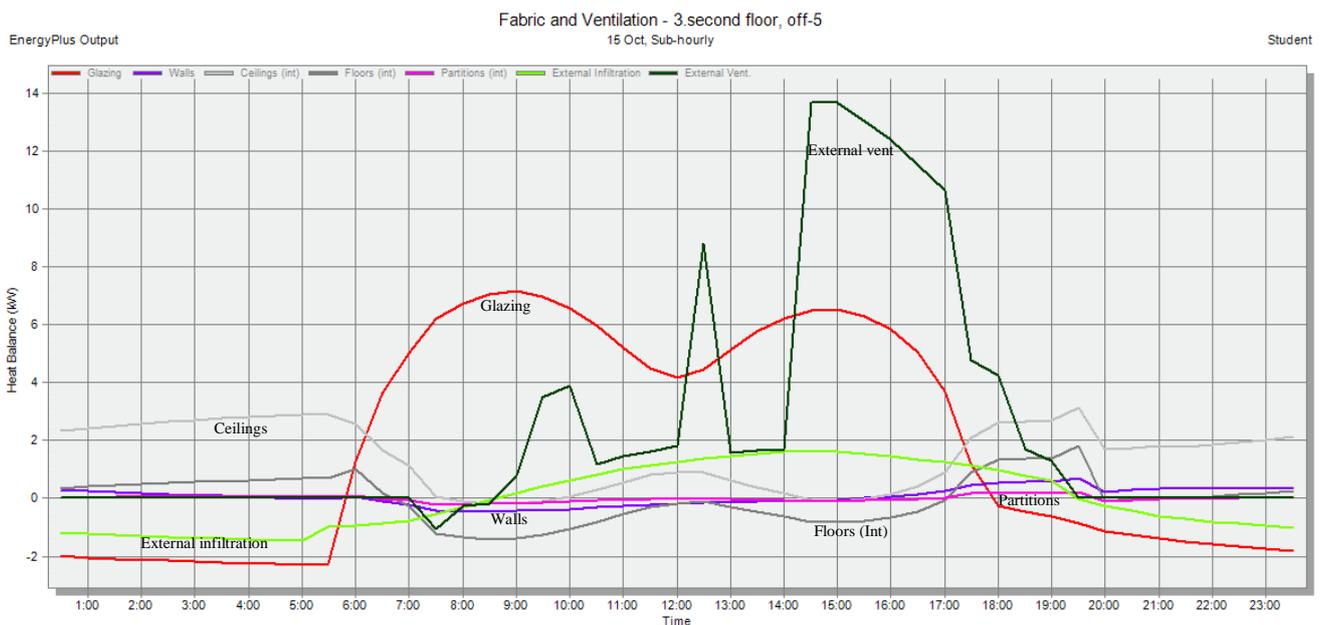
Figure 37: Example of north facing zone-Office 4 (red line shows glazing –peak 2.51kW). Offices 2, 6, 7 follow a similar profile
