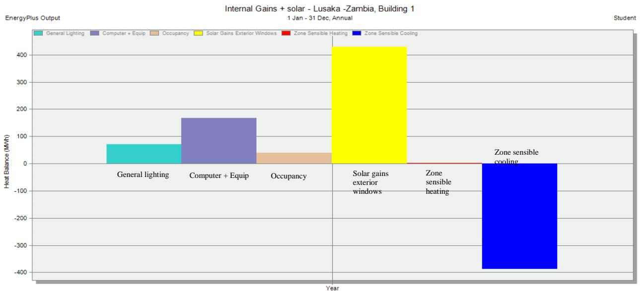
Figure 31: Internal gains breakdown and sensible cooling.
