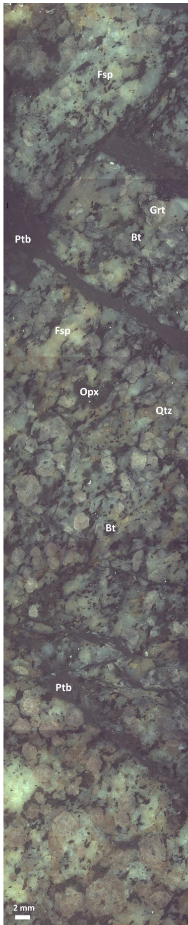
Figure 2.5: SK4A. Garnet-orthopyroxene-biotite-bearing stromatic metagreywacke from the farm Jagers Vrede. Dark-grey, cryptocrystalline pseudotachylitic breccias (Ptb) crosscut the sample forming a fine, interwoven mesh in places.
