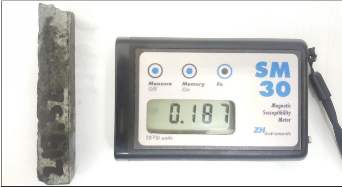
Figure 3.23: SM-30 Magnetic susceptibility meter alongside pyroxenite quarter-core displaying susceptibility reading.
