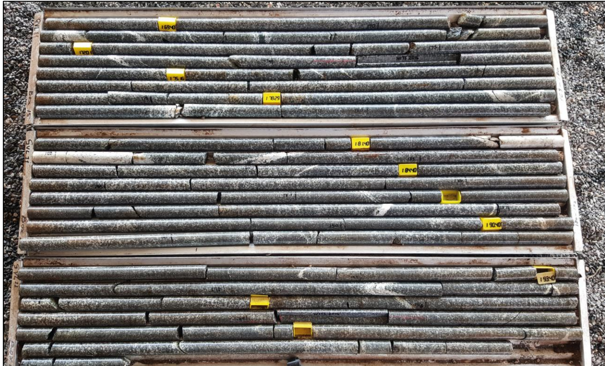
Figure 3.9: Norite package intersected in borehole GVL 2 cut by several quartzofeldspathic veins.
