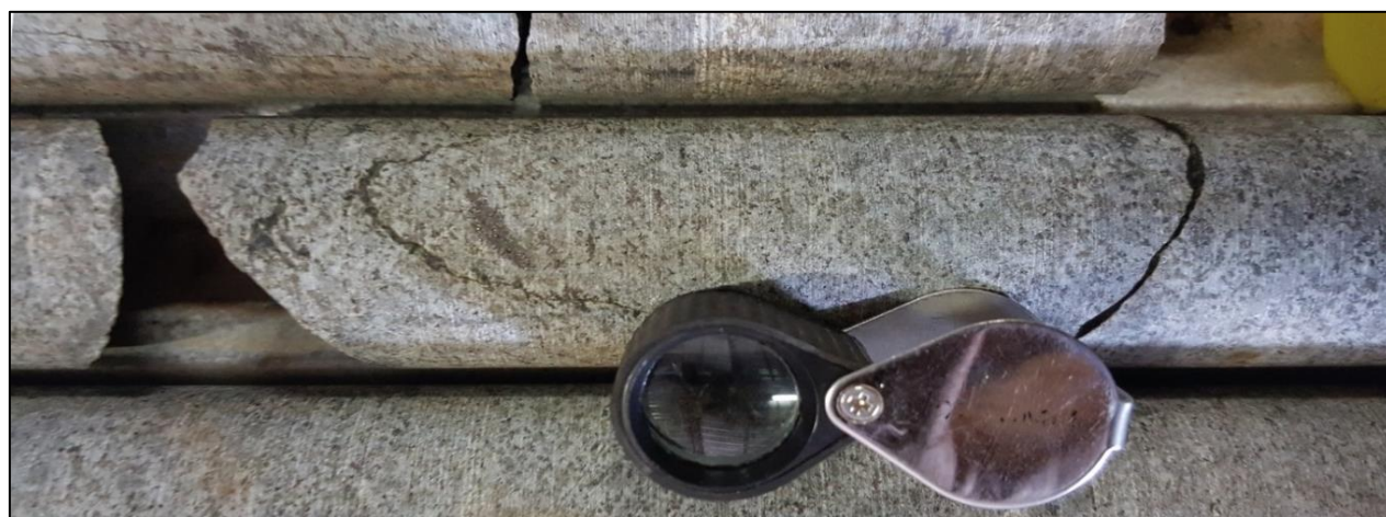
Figure 3.11: Fine-grained magnetite bleb within norite intersected in borehole GVL 2.
