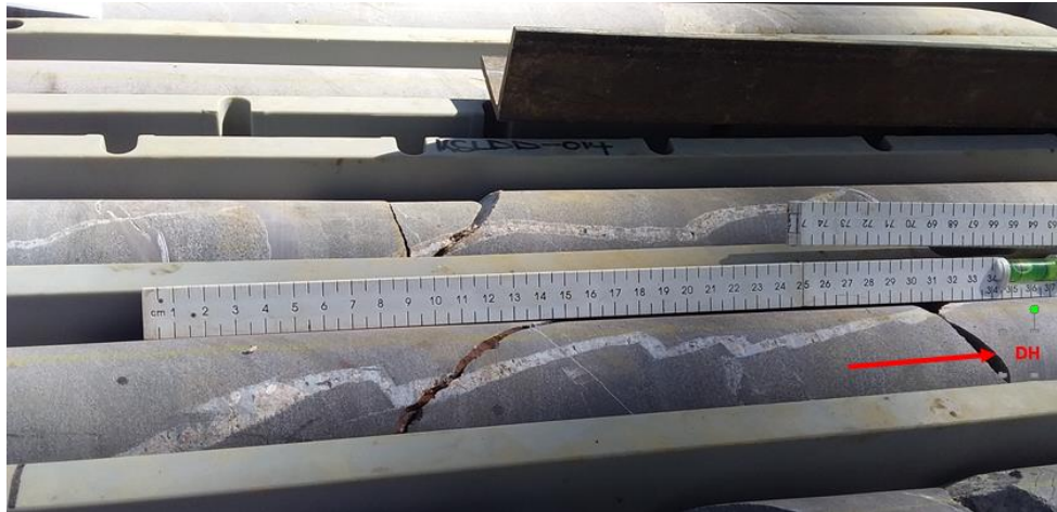
Figure 22. Z-folding marked by quartz vein in arkosic sandstone unit, from drill hole DDH0014. DDH drilled at location UTM Arc 1950 210,074mE/8,688,900mN. Red arrow pointing in the downhole direction.
