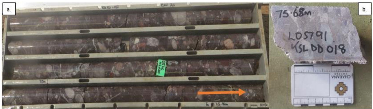
Figure 10. Borehole core tray of the conglomerate unit. (a) Photograph of conglomerate unit from diamond drill core with HQ core size sampled from hole ID DDH0018. Arrow points in the downhole direction. (b) hand size sample of the analysed drill core collected at depth 75.6 – 75.80 metres.
