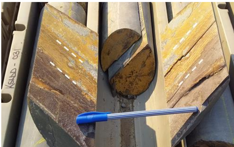
Figure 26. Slickenlines (marked by white dotted line) on slickenside surfaces with FeOx coating on surface. Pen for scale (~15cm)
