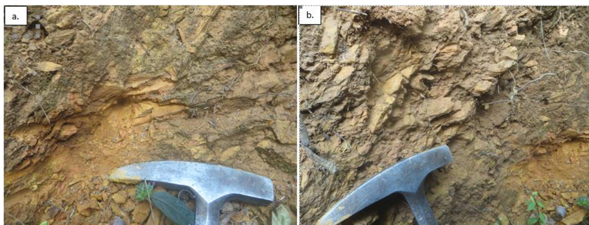
Figure 8. Exposure of the Roan shale in an exploration trench showing (a) weathered saprolitic shale with FeOx alteration (b) weathered saprolitic shale in historical exploration pit at location UTM Arc 1950 Zone 35 South 208912mE/8688760mN with relics of bedding.
