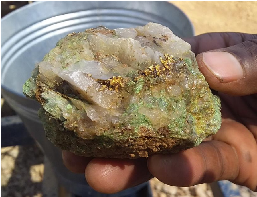
Figure 31. Hand-size sample showing a gold mineralised quartz vein from the diamictite – arkosic sandstone – quartz vein contact zone, with green chlorite staining from the diamictite unit.
