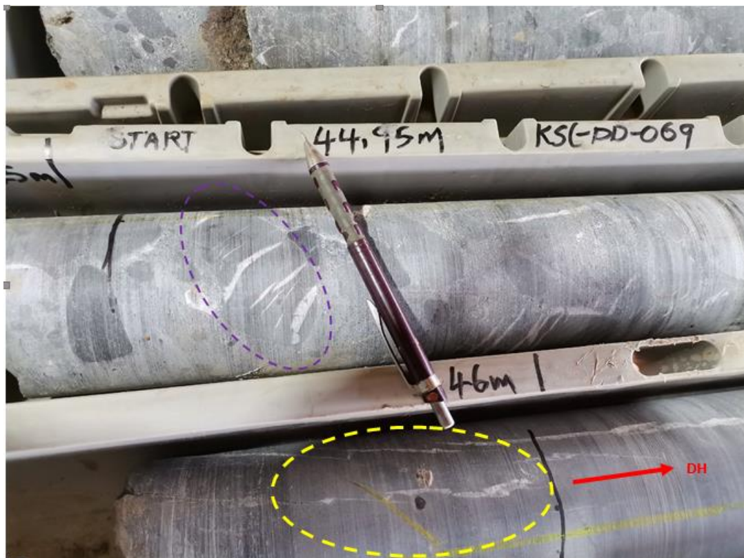
Figure 24. Photograph of diamond drill core from hole ID DDH0069. Clast rich diamictite unit (“Grand Conglomerat” marker bed), with sheared pebble size clast (marked by dashed purple ellipsoid circle) and calcite filled tensional fractures oriented perpendicular to the shear direction. Note the S-type of parasitic folds at 46.00m. Pencil (~15cm) used for scale and red arrow pointing in the downhole direction.
