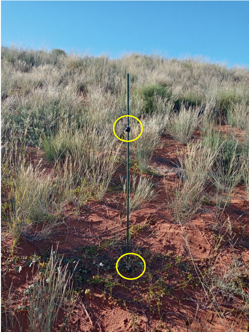
Figure A3.10. An example of one of the ‘exposed site’ macroclimate loggers in the dunes. Temperature loggers at ground level and above-ground level are encircled in yellow.
