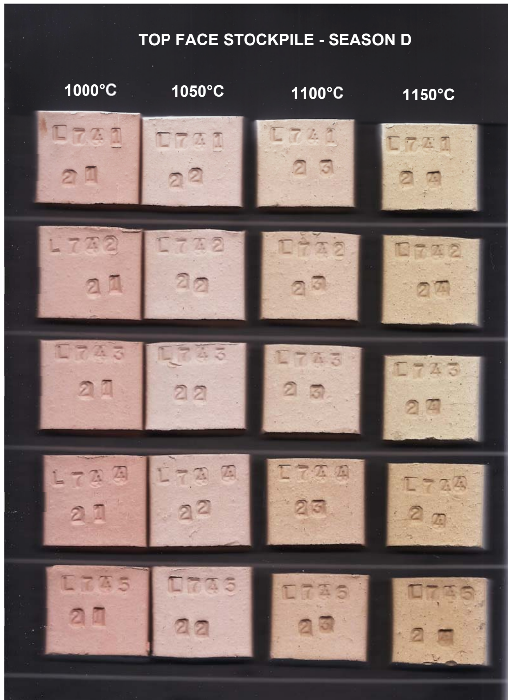
Figure 1-12. Fired briquettes for season D stockpile, showing colour development over a temperature range of 1 050 °C to 1 150 °C. Variability in colour of the briquettes for each temperature at different positions is insignificant.
