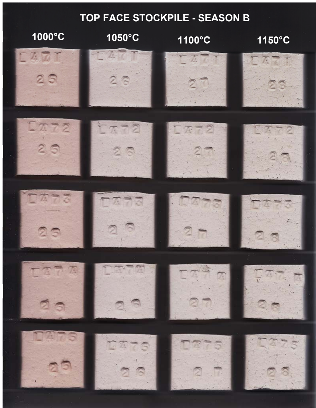
Figure 1-10. Fired briquettes for season B stockpile, showing colour development over a temperature range of 1 050 °C to 1 150 °C. Variability in colour of the briquettes for each temperature at different positions is insignificant.
