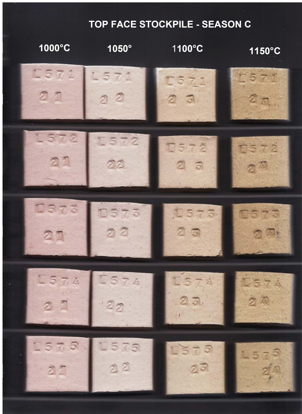
Figure 1-11. Fired briquettes for season C stockpile, showing colour development over a temperature range of 1 050 °C to 1 150 °C. Variability in colour of the briquettes for each temperature at different positions is insignificant.
