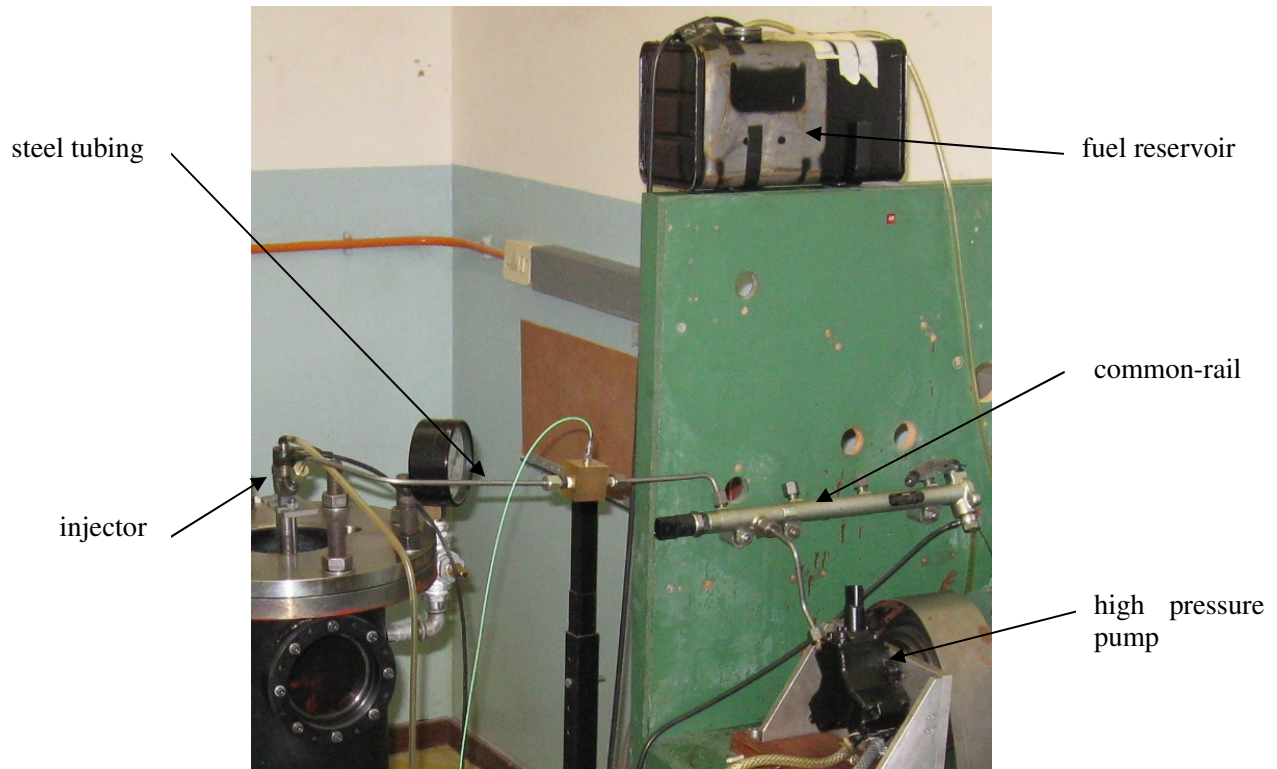
Figure 21: Common-rail system.
