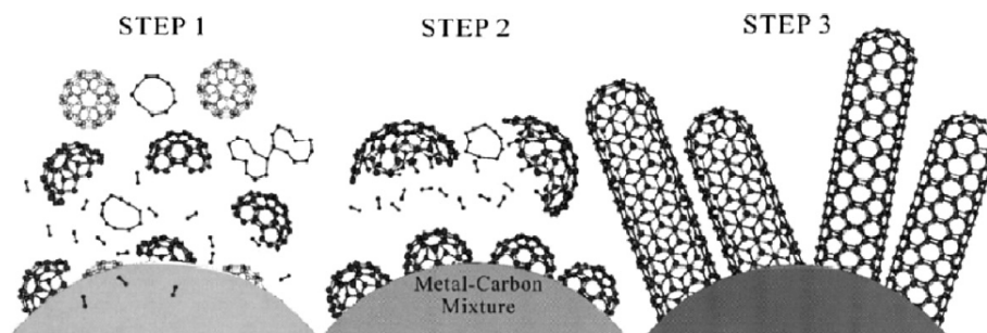
Figure 2.12: S-L-V mechanism put forward by Kautara et. al. showing that the growth of SWCNT is preceded by fullerene like seed. Taken from Ref. [51].
