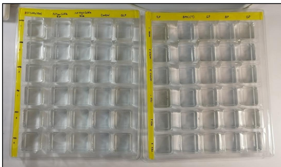
Figure 3.2: An example of the layout of each 30-well test plate used for the Daphnia magna test. The different patches/interpatches for each pollution zone are along the length of the plate, while fed and unfed wells occur along the width of each plate. The three wells per fed and unfed sections comprised the triplicate leachate solutions for each patch/interpatch.
