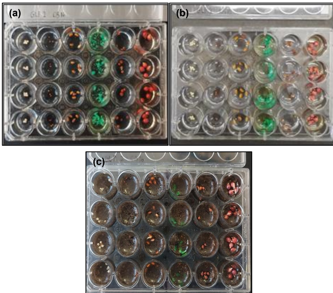
Figure 4.2: Filled repli-dishes containing seeds with (a) FLP solutions, (b) SPLP solutions, and (c) soil samples.
