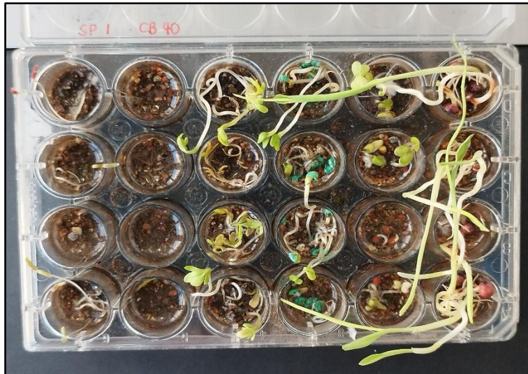
Figure 4.3: Example of a repli-dish containing seeds placed directly on the soil test sample.
