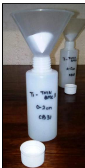
Figure 2.6: Leachate extraction method using ash-free non-adsorbent Millipore water filter paper and a plastic funnel.
