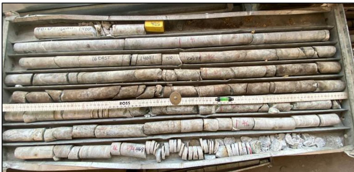
Figure 36: Shows Highly jointed rock mass with discing at HD 14051 from 40m-47m
