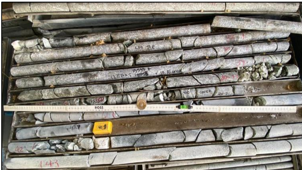
Figure 39 Shallow dipping joints with mechanical drilling break HD 14072 from 35-42m
