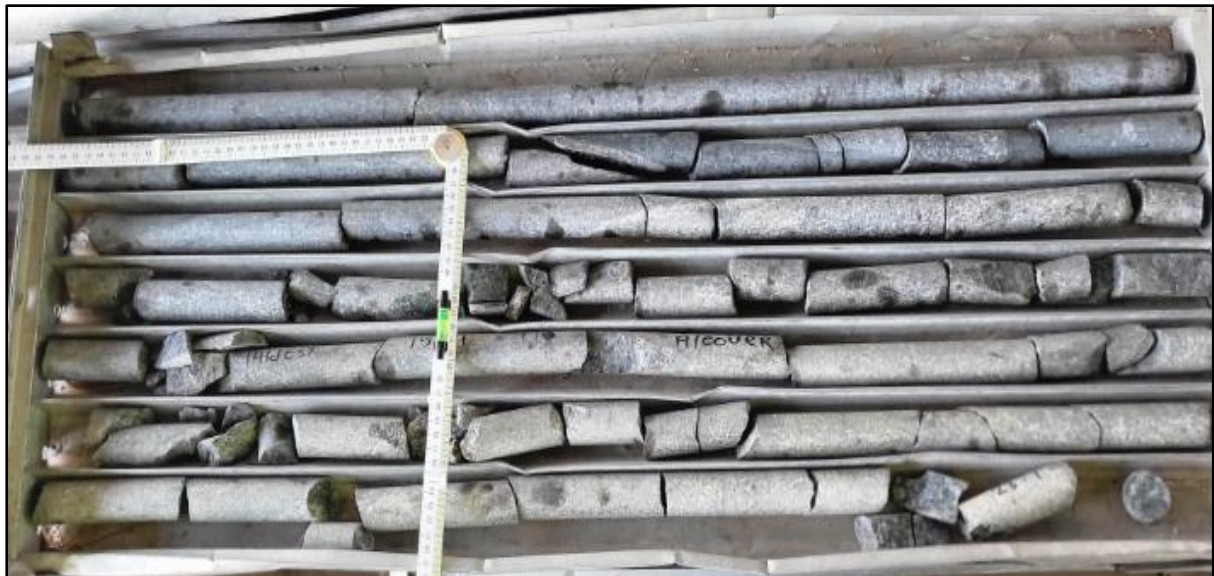
Figure 32: Borehole HT030 drilled, moderately weathered joints were recorded at Borehole HT030 from 24-28.4m.
