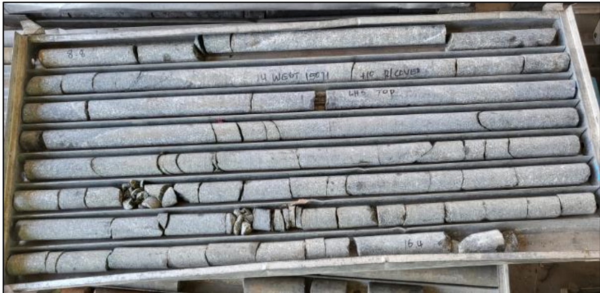
Figure 33: Shows Borehole HT030 drilled, with some areas with disc failure at the core at Borehole HT030 from 8.8-16.4m.
