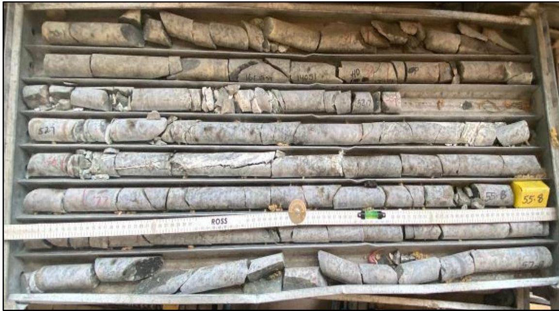
Figure 35: Shows HD 14051 borehole number from 16 FDE with shear zones seen at the core at HD 14051 from 50.1-57.8m
