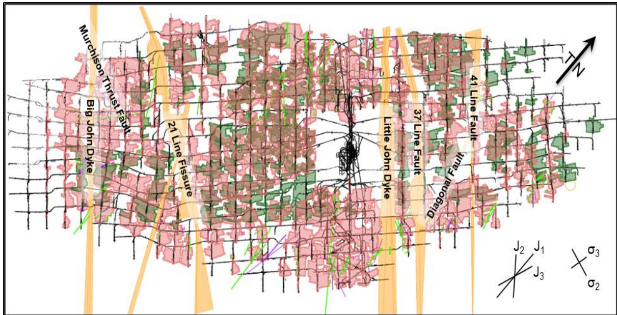
Figure 5: Plan depicts water pillars in orange on major geological structures with Merensky stopes (red) and UG2 stopes (green). (Zondereinde Mine COP, 2024)
