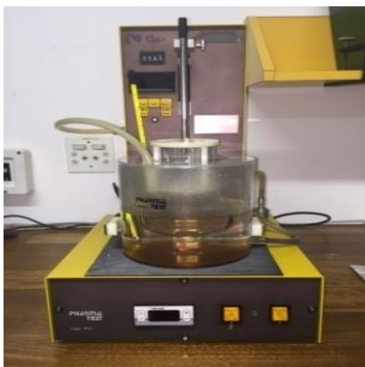
Figure 4.4: The Modified Disintegration Apparatus that was used for Testing Disintegration Time.
