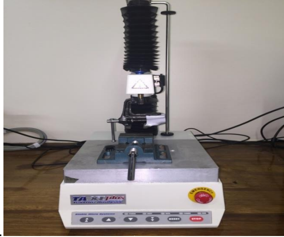
Figure 4.3: The Texture Analyzer was used for measuring Tensile Strength.
