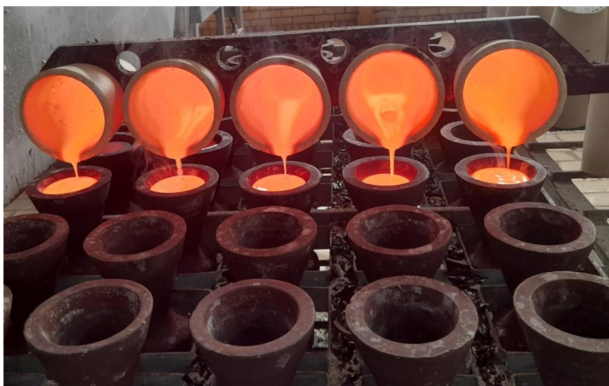
Figure 5.1 Pouring of the fused sample into iron molds.
