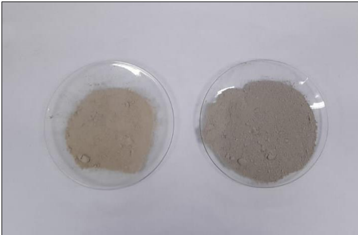
Figure 5.4 The tailings materials used for the study. Left (VCR matrix) and right (GSB matrix).
