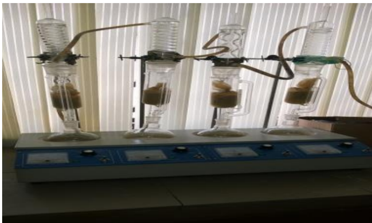
Figure C.2: Oil soxhlet extractor used for the study
