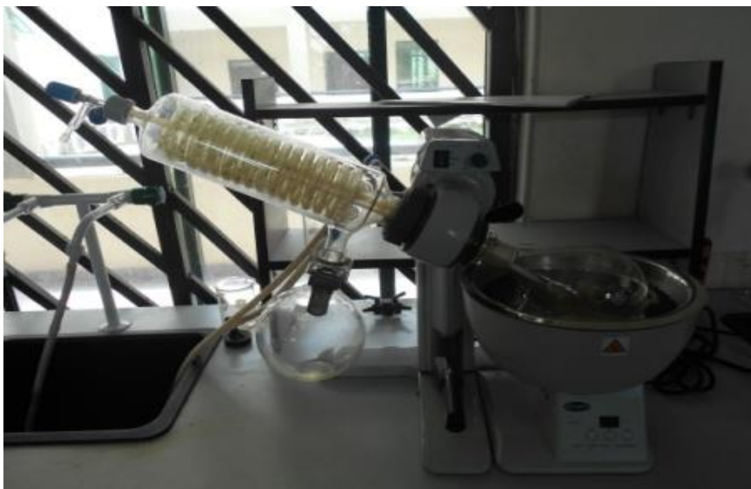
Figure C.3: Rotary evaporator used in the study
