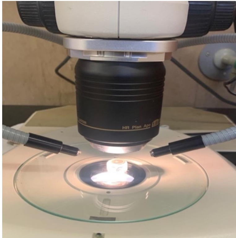
Figure 6: Failure mode being assessed on a PEEK specimen using a Stereo Microscope
