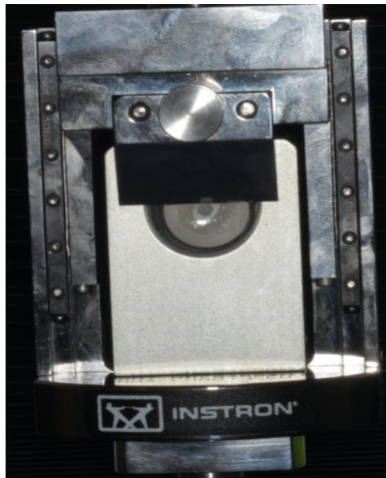
Figure 5: PEKK specimen securely contained within the stainless-steel frame of the Instron universal testing machine. A chisel-shaped rod fitted with a 2kN load cell directed at the adhesive interface
