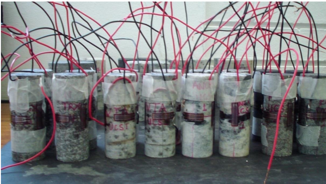
Figure 3.5: Specimens with strain gauges and lead-wires
