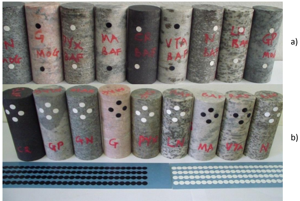
Figure 3.35: Rock specimens with markers for a) axial and b) transverse thermal strain measurements
