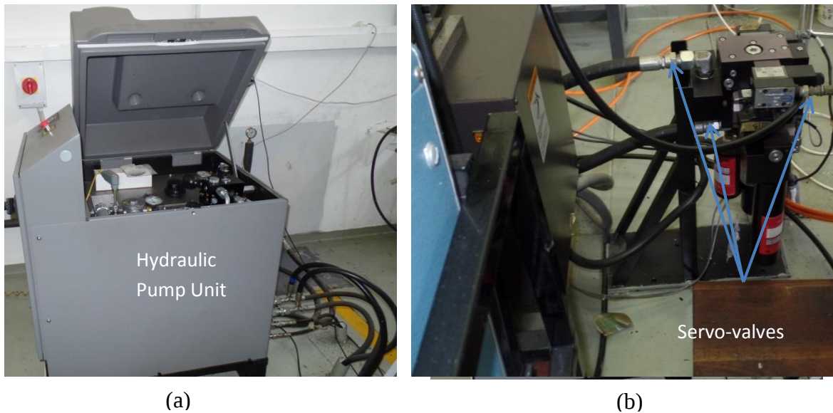
Figure 2.29: Servo-controlled machine support systems (a) Hydraulic Pump Unit (b) Servo-valves
