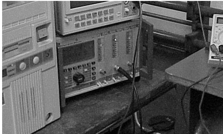
Figure 4.21: Strain gauge signal conditioner and power supply.
