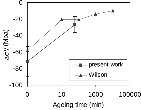
Figure 7.2: Rise in reverse yield, \Delta\sigma_y , with ageing time, a comparison with Wilson and Ogram's results [4].
