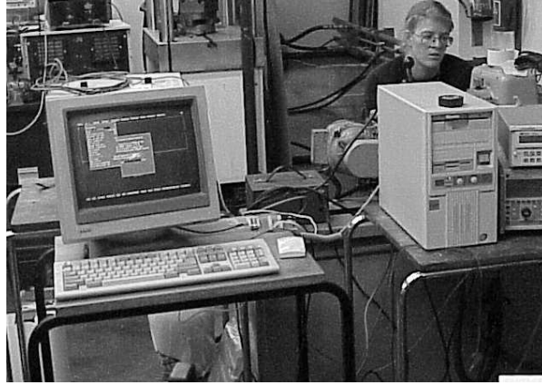
Figure 5.4: 486 Computer with wave view software and PC30D board.
