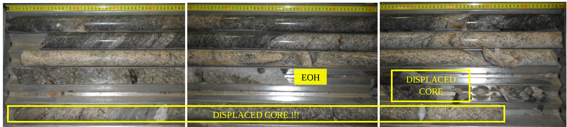
Box 33 , Box depth = 363.48 -368.58 m (End of the M4 drillcore)
