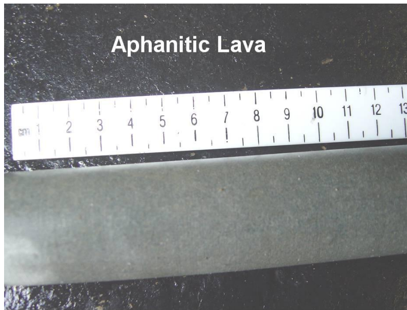
Figure 2.4: Photo of an aphanitic lava rock sample from a drill core
