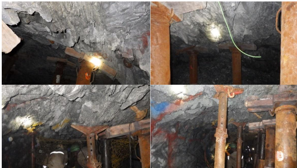
Figure 4.4: Photos from different stopes showing the uneven hangingwall conditions in the west mine stopes
