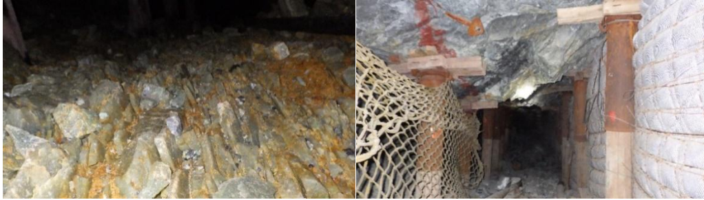
Figure 4.5: Uneven footwall conditions created by the hard and brittle quartzite rock mass
