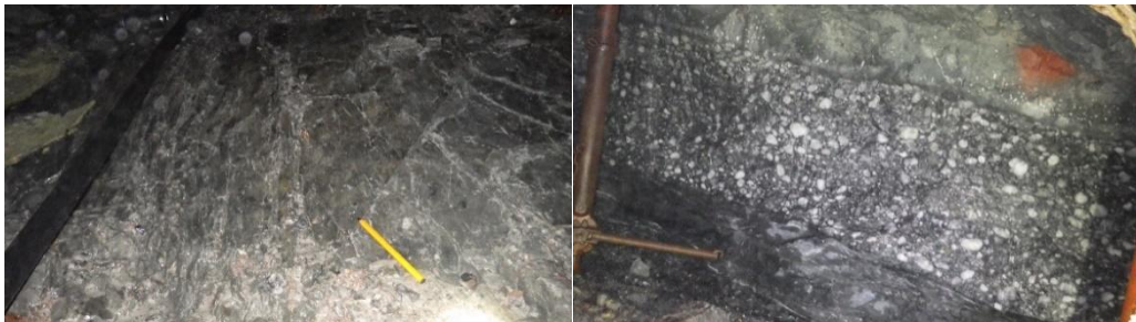
Figure 4.3: Smooth footwall conditions created by the soft shale rock mass
