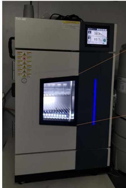
Figure 7.1: Equipment used for determining the optimal temperature that can be used to immobilise adult sterile males: A 25 ℓ climate chamber (Jeio Tech, model: TH3-ME-025, South Korea) with a transparent cylindrical plastic cup covered with an elastic band secured fabric net inside which mosquitoes were aspirated and through visual observation knockdown time recorded.
