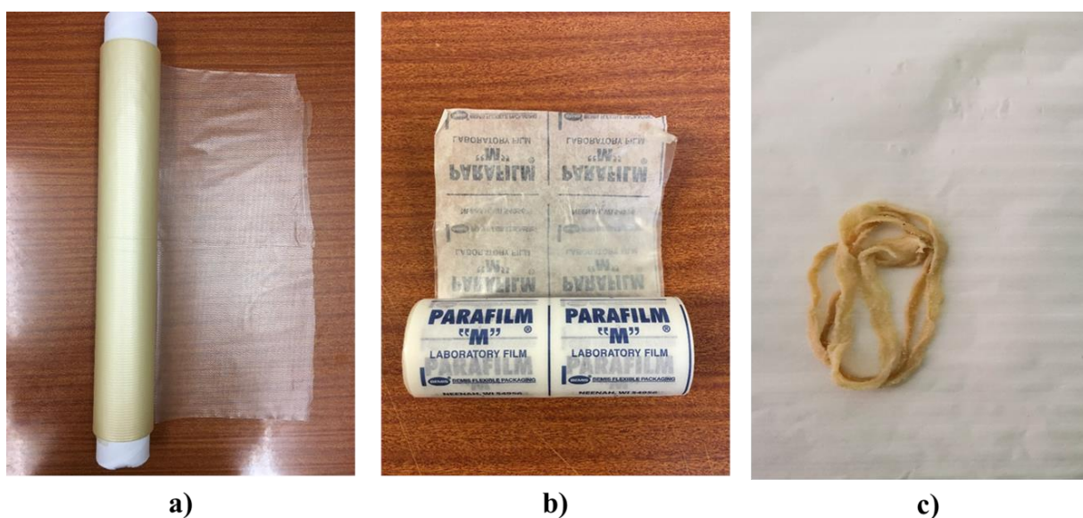
Figure 2.2: Artificial membranes used in this study during blood feeding optimisation of a laboratory An. arabiensis colony: (a) Collagen membrane (dimensions: 580 mm wide × 30 m length, thickness: 10 to 20 µm), (b) Parafilm-M ® (dimensions: 101.6 mm wide × 100 m length, thickness: 10 to 20 µm), (c) Hog casing (dimensions: 28 mm wide × 20 m length, thickness: 10 to 20 µm)
