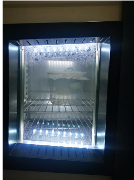
Figure 7.1: Equipment used for determining the optimal temperature that can be used to immobilise adult sterile males: A 25 ℓ climate chamber (Jeio Tech, model: TH3-ME-025, South Korea) with a transparent cylindrical plastic cup covered with an elastic band secured fabric net inside which mosquitoes were aspirated and through visual observation knockdown time recorded.
