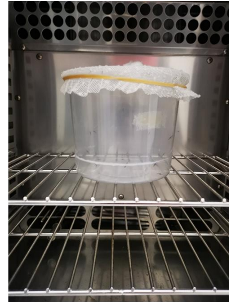
Figure 7.1: Equipment used for determining the optimal temperature that can be used to immobilise adult sterile males: A 25 ℓ climate chamber (Jeio Tech, model: TH3-ME-025, South Korea) with a transparent cylindrical plastic cup covered with an elastic band secured fabric net inside which mosquitoes were aspirated and through visual observation knockdown time recorded.
