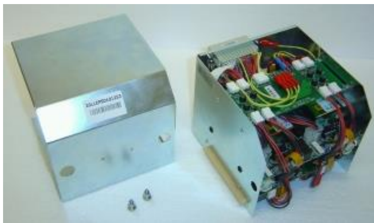
Figure 3.1: LVPS box assembled.
