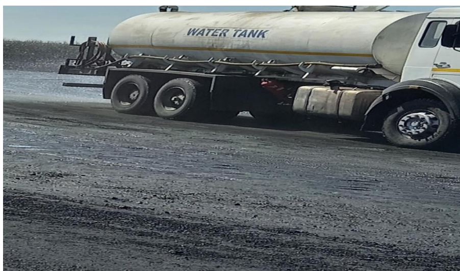
Figure 5: Typical coal dust suppression method using 1800L water tanker.
