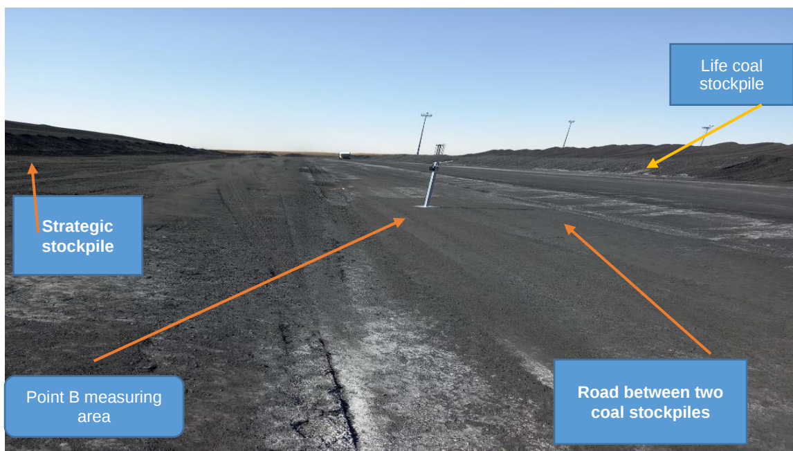
Figure 9: Typical coal dust measuring instrument placed at Point B (between 2 stock piles).
