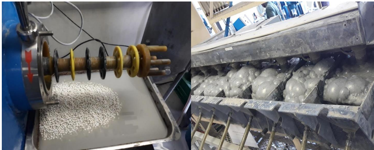
Figure 3.1: Grinding disk and shaft of M4 IsaMill and flexi-float flotation cells
