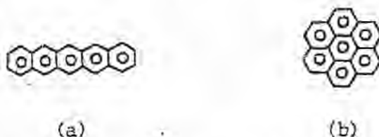
FIG 12 : NATURE OF THE "COKE" FORMED EXTERNALLY ON a) ZEOLITE Y AND b) H-ZSM-5 DURING THE CRACKING OF n -HEPTANE [1.37]
