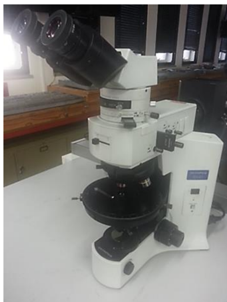
Figure 5.1: Olympus BX41 petrographic microscope at the petrography laboratory, University of the Witwatersrand School of Geoscience, 2017
