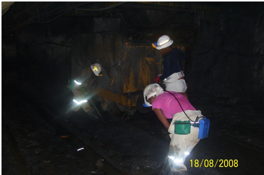
Picture: Female workers removing ore from the drain and loading it onto a hopper
