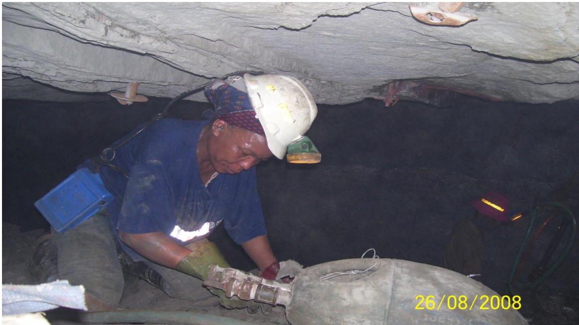
Picture: A female worker preparing a water pump inside a stope
