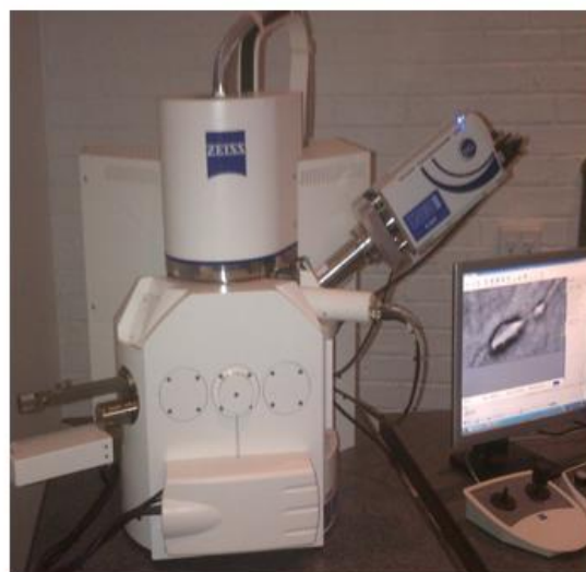
Figure 6: Key components of SEM instrument (Skoog et al., 2014)
