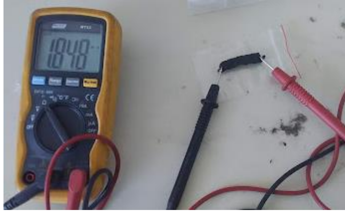
Figure 11: Multimeter for measuring resistivity of the sample
