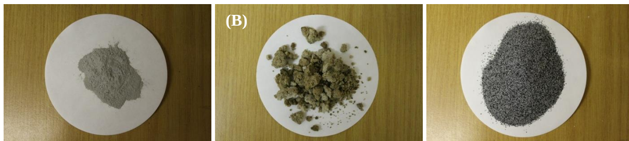
Figure 3-2 As received (A) South African coal fly ash (B) pulp waste (C) pulp waste ash
