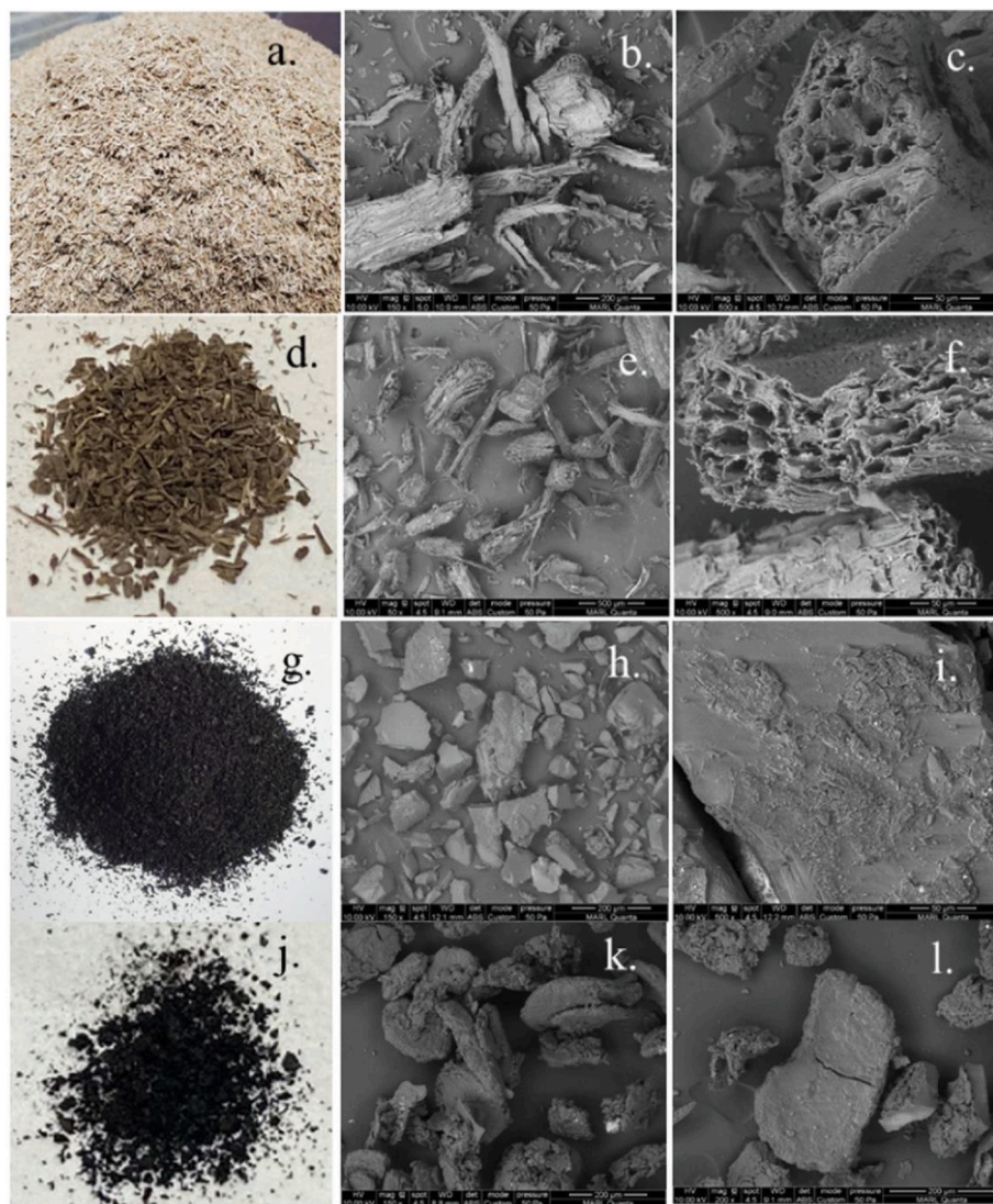
Fig. 4. SEM images of a-c. Red oak feedstock, d-f. Pretreated red oak feedstock, g-i. Solid char result from co-pyrolysis of red oak and polyvinyl chloride (PVC) ratio 1:1, j-l. solid char result from co-pyrolysis of red oak and PVC ratio 2:3 [172].
